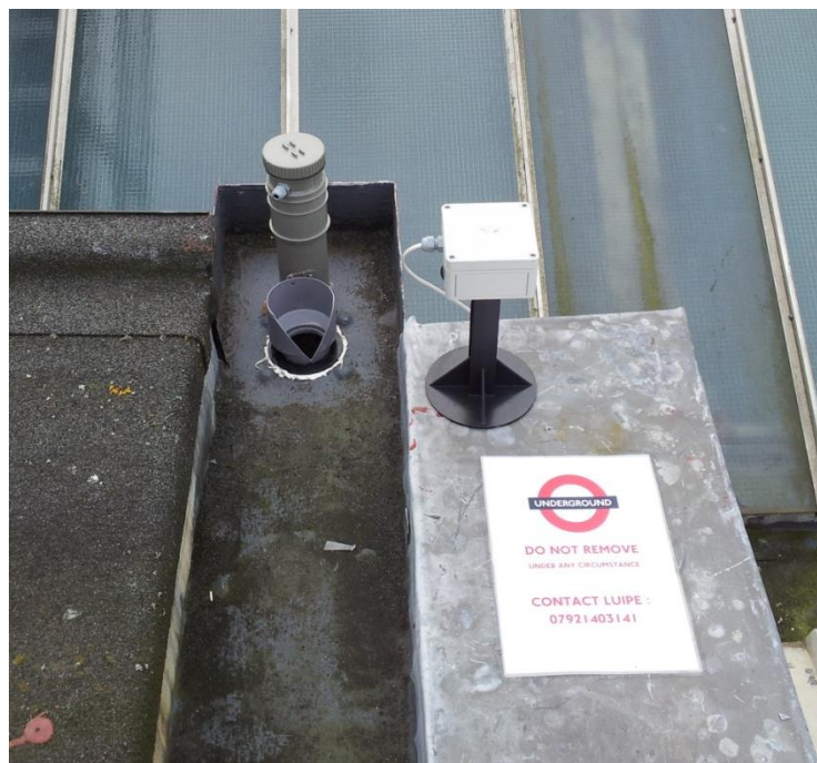
Figure 2. V-notch capacitance sensor monitoring device.
