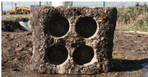
Fig 3: 1:1 sample achieving 32% concrete saving utilising locally available material
