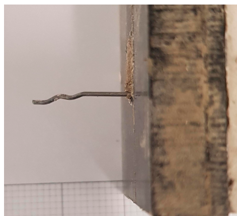
Figure 8. The 5D hook not being fully straightened following the pull-out test.
