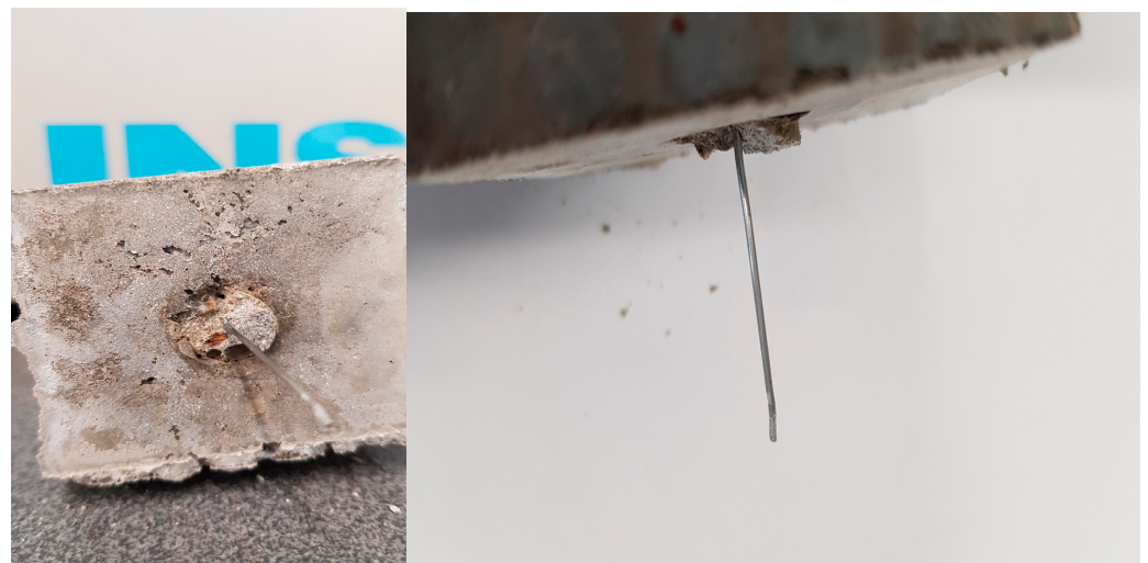
Figure 6. The pull-out specimen at the end of testing.
