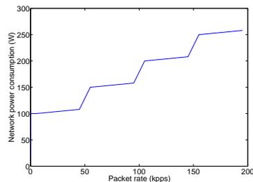
Fig. 4 Step-like router power profile used in the experiments
