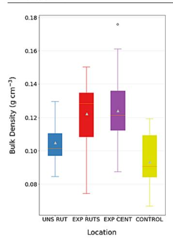
**FIGURE 4** Boxplots comparing bulk density for the four sampled locations. The mean and median are represented by the grey triangle and orange line, respectively, box ends represent IQ1 and IQ3, whiskers represent values up to 1.5 times the IQ range with fliers representing the extreme outliers.
