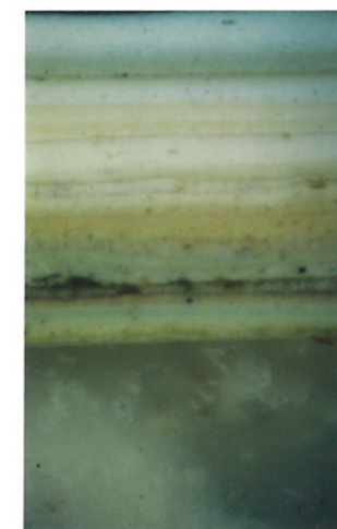
Plates 26 & 27 (right). Close examination of Sample 29, taken from the background of the monogram inside the foliate wreath, indicates that this area was initially painted a pale green colour, but that this was swiftly changed to a pale pink to match that outside the wreath but inside the octagonal moulding (Sample 28, Plate 25). Plate 27 (far right) shows the original scheme at greater magnification, with the pink lying directly over the pale green. The zone just outside the octagonal moulding remained a pale green colour (Sample 18). (Photomicrographs: Howard 1997)
