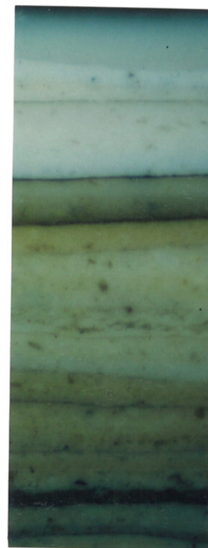
Plate 15 (left). Cross-section of Sample 48, taken from the background of the raised decoration of the architrave of the southwest door. Unfortunately, the lowest (original) paint layer is barely visible in the photomicrograph, but a single black particle at bottom right is indicative of a layer which consists of charcoal black in a white matrix. The overall appearance is likely to have been a pale grey colour. The support here is wood (again missing in the cross-section). Plate 16 (above) Cross-section of Sample 47, taken from the raised decoration on the architrave. The original paint-layer here would have been creamy white in appearance. The contrast provided by the pale-grey shadowing (Sample 48, Plate 15) would have enhanced the relief of the ornament. (Photomicrographs: Howard 1997).
