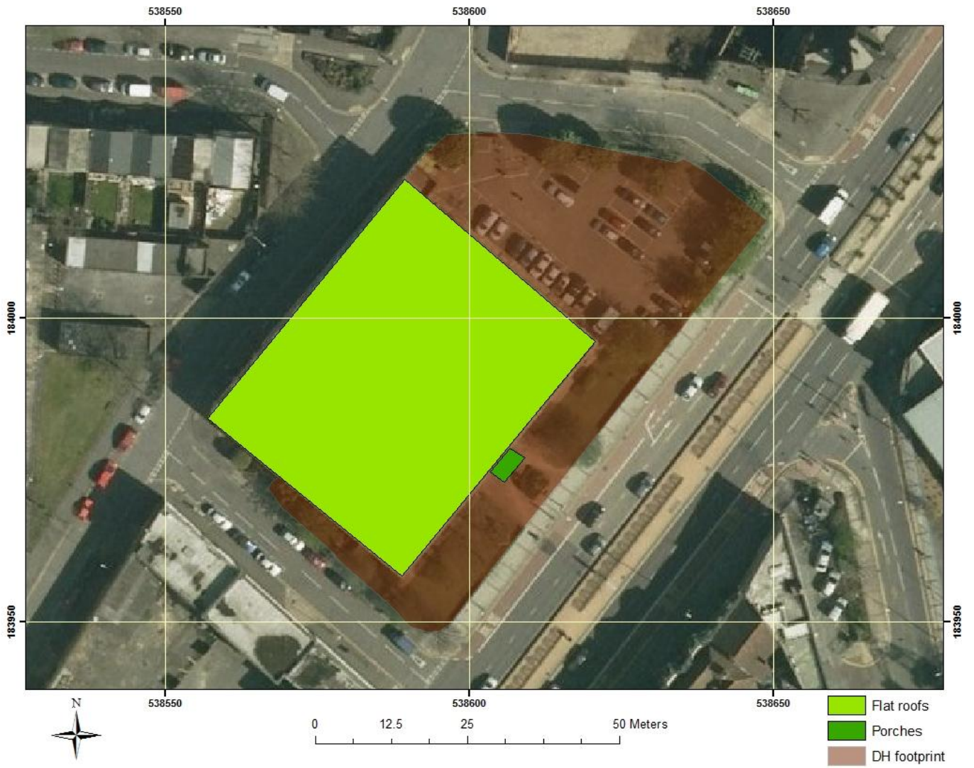
Figure 8: Duncan House featured a large flat roof on the single building, with a small porch. This comprised potential for a retro-fit green roof. Aerial photograph backdrop © Getmapping.com
