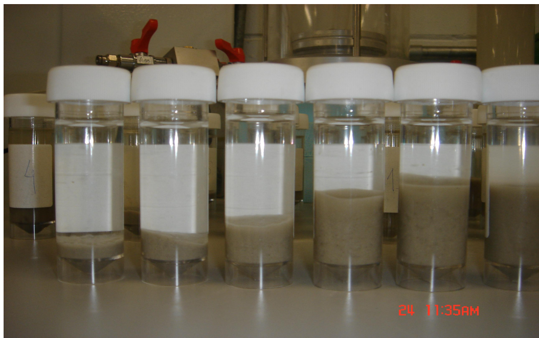
Figure 4 – Free swell of clay liner infill in sea water (left) and deionised water (right)
