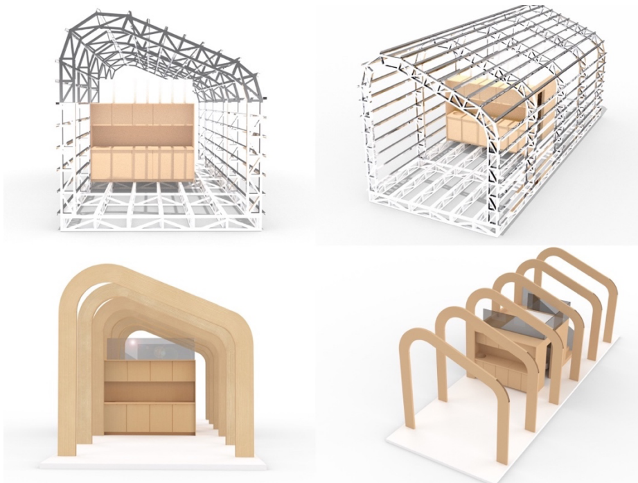
Figure 5. Elemental House design exploration options allow different structural systems. 3D Printed physical models. Source: D. Benros et al, 2023.
