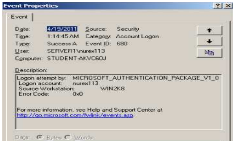
Fig. (5.3): Event ID 680 recorded when the attacker successfully guessed and logon with the user account nurex113.
