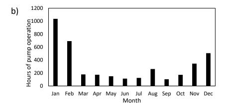
**Figure 4.3** a) Water fluxes for Redmere Farm (EF-SA) in 2014 showing how the balance of precipitation and evapotranspiration must be lost as discharge (notably in winter; Source: **Evans et al., 2017**). b) Pump operation at Lark station for 2014 showing how pumping operations are most intensive in winter periods
