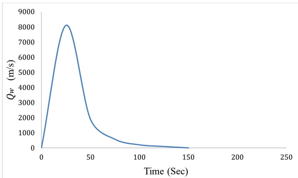
Figure 3.6 Calculated breach hydrograph
