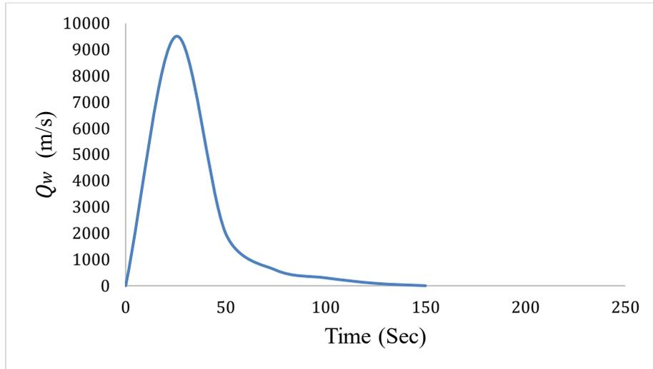
Figure 3.5 The HCE-RAS 5.0.7 produced breach hydrograph
