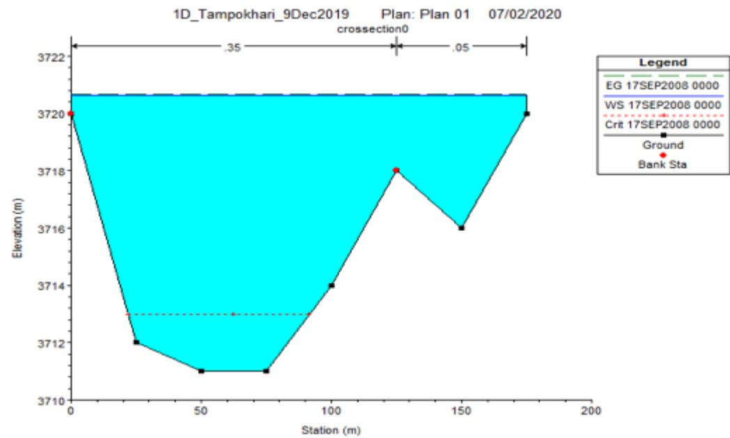
Figure 3.9 Flooded River station at Inkhu river due to GLOF
