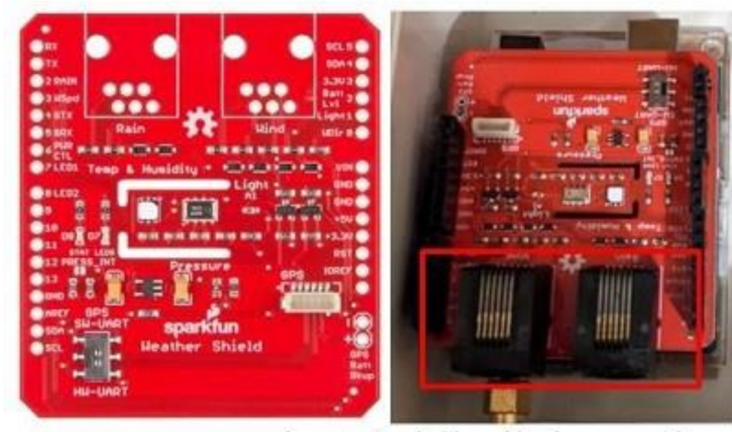
Figure 3. Installed SparkFun weather shield
