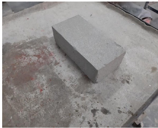
Fig. 9: A typical cured CSEB (Elahi et al. 2020)
