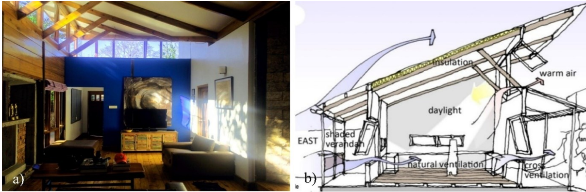
Fig. 13: Nel Sedone house living-room after adaptation to cold-cloudy Shillong, (a) afternoon solar heat gain from South, West glazing and absorption with thermal mass walls and interior elements, (b) section of daylight heat gain and ventilation (Gupta et al. 2023).
