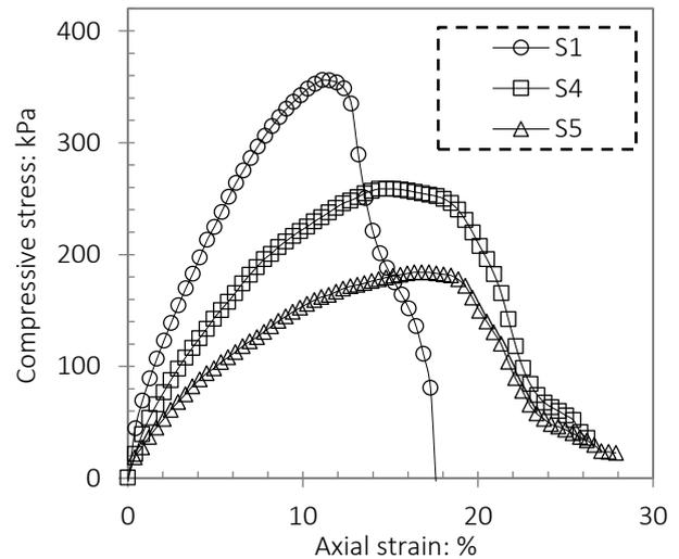
Fig. 3 Stress-strain patterns from unconfined compressive strength experiments
