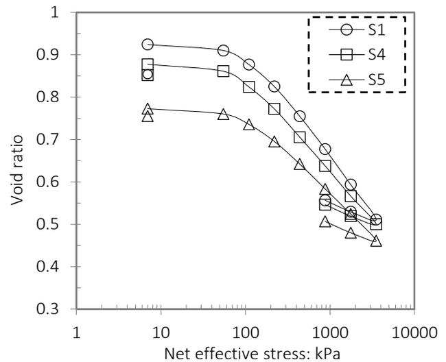
Fig. 5 1D consolidation  $e$ - $\log \sigma'$  curve
