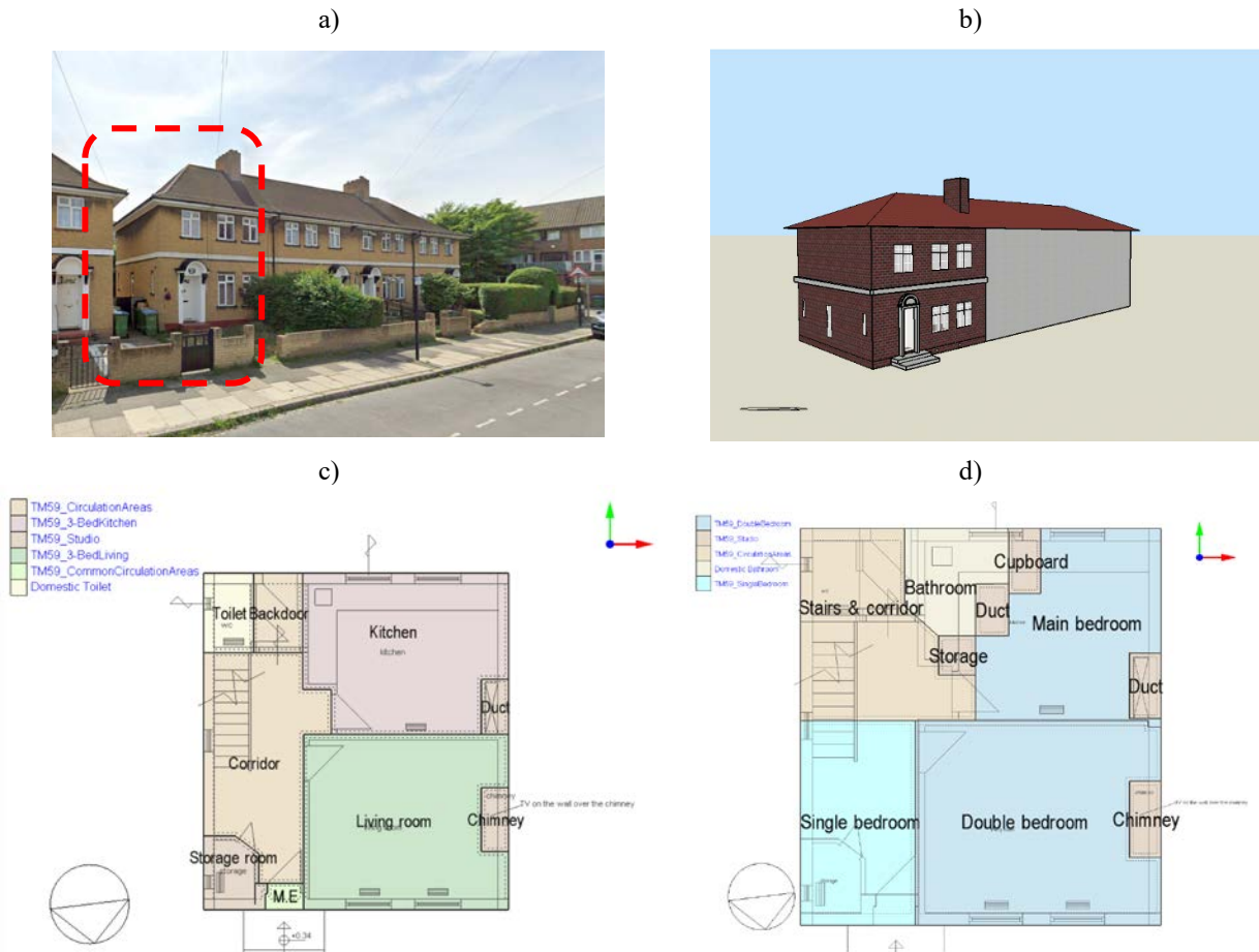
Figure 2: (a) a picture of the case study house. (b) the 3D model of the case study house. (c) Ground floor plan. (d) First floor plan (by the Author).
