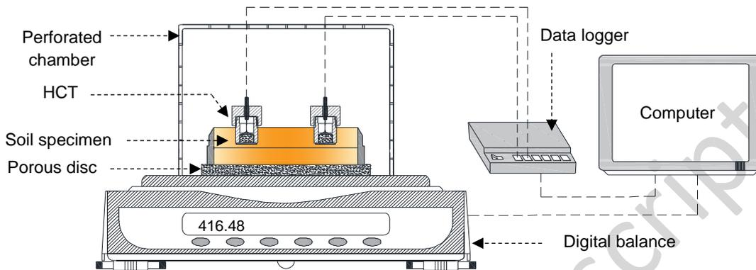
**Figure 2.** Schematic drawing of the experimental setup for SWRC measurement
