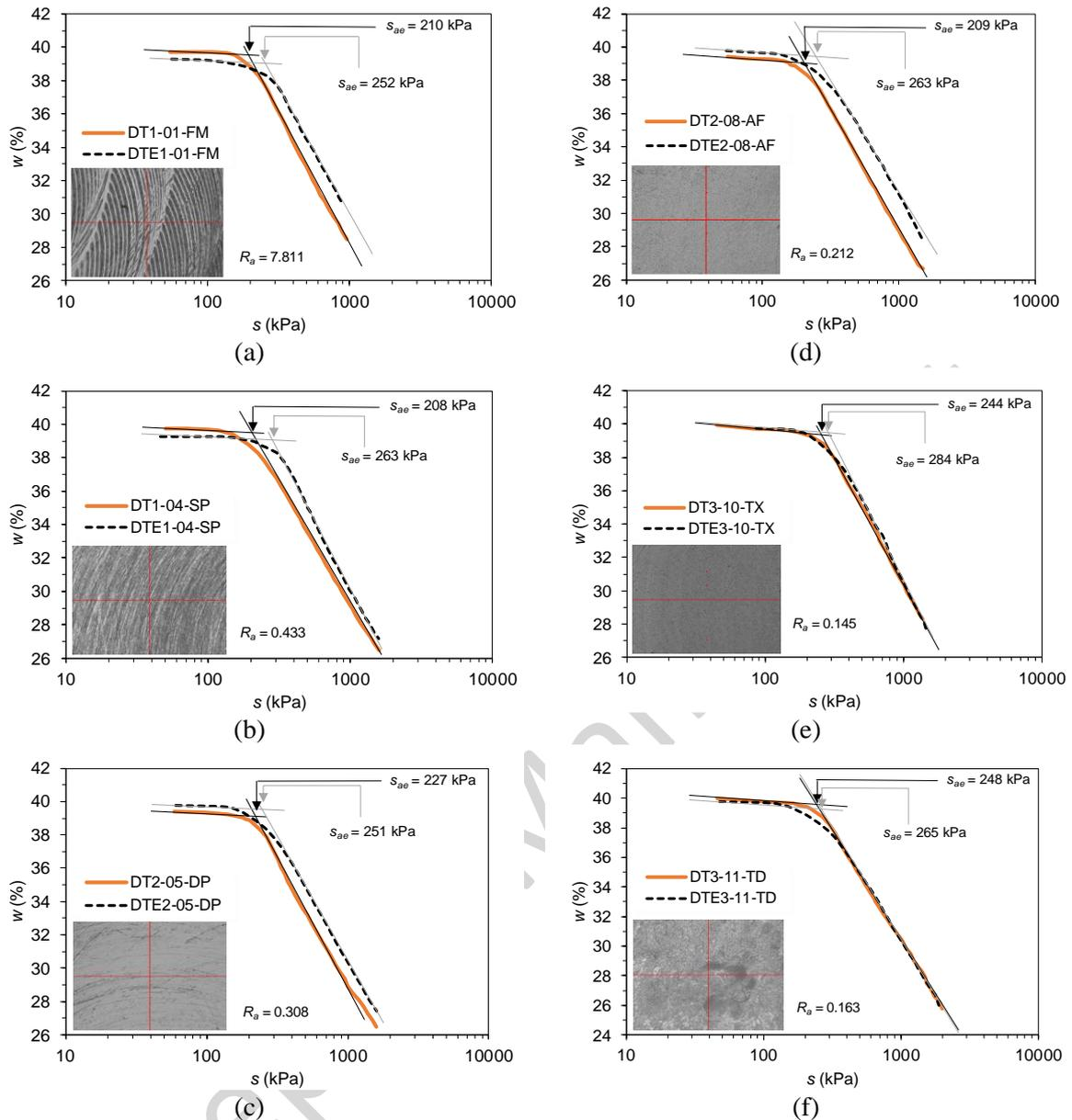
**Figure 6.** Comparison of SWRCs obtained from DT and DTE tests for different HCT types: (a) FM; (b) SP; (c) DP; (d) AF; (e) TX; and (f) TD
