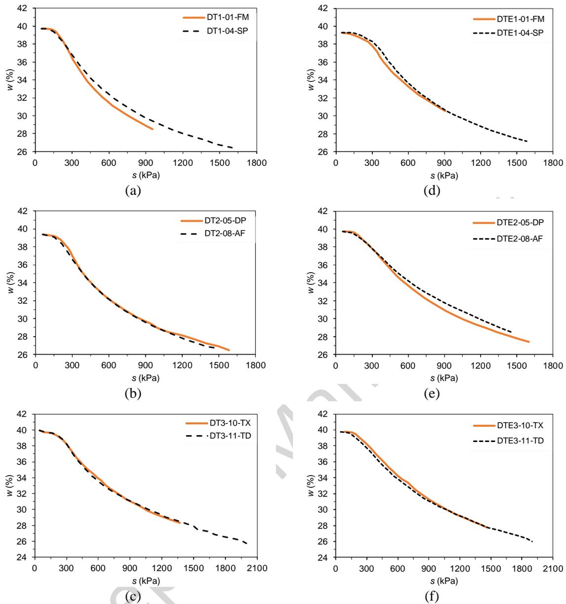
**Figure 5.** SWRCs obtained from HCT measurements: (a) DT1; (b) DT2; (c) DT3; (d) DTE1; (e) DTE2; and (f) DTE3
