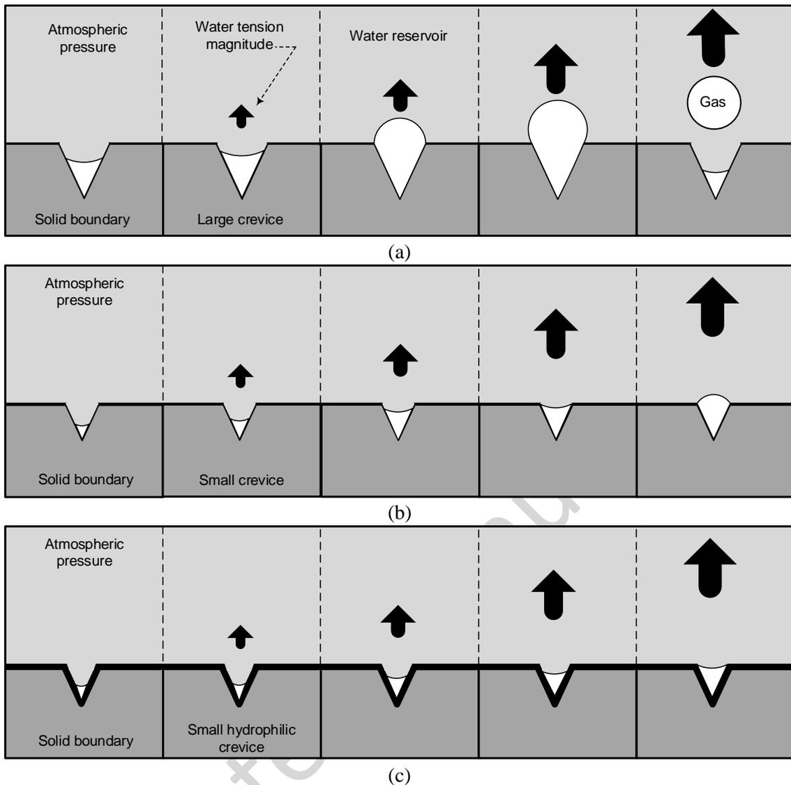
**Figure 12.** Cavitation inside the water reservoir: (a) large crevice; (b) small crevice; (c) small hydrophilic crevice
