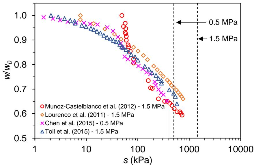
**Figure 8.** Drying-path SWRC of fine-grained soils determined using HCTs and following continuous drying method
