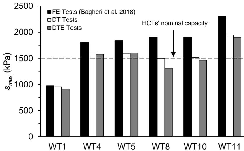
**Figure 7.** Performance of HCTs in terms of  $s_{max}$  during FE, DT, and DTE tests
