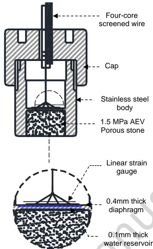
**Figure 1.** Schematic diagram of WT and its components
