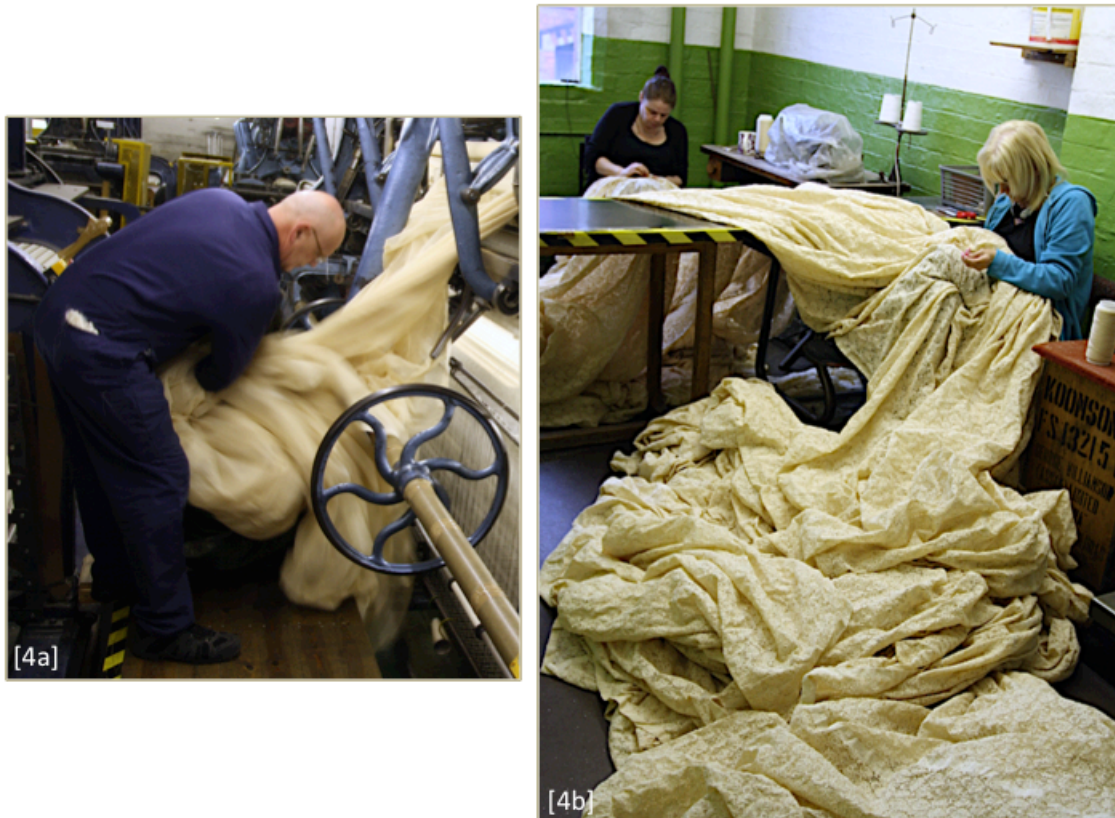
Figure 4. (a) Removing the lace ‘web’ from the machine, ready for mending and (b) group mending to repair an extensive flaw.
