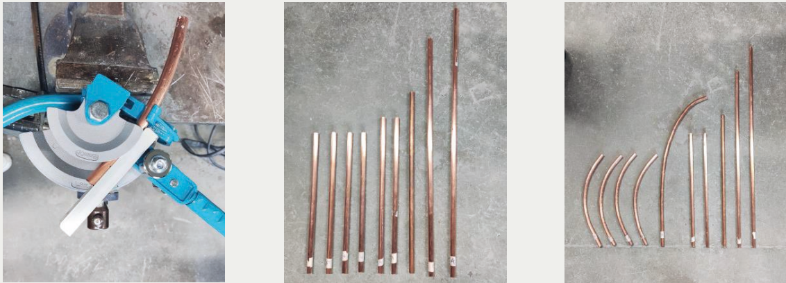
Figure 6. Analog pipe bender and using a segmental making to bend pipe to template and individual radius.
