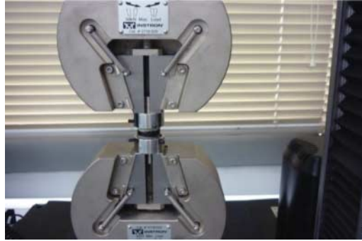
Figure 2. Adhesion strength test set-up.
