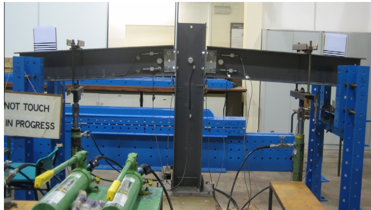
Fig. 12. Excessive joint rotation ( \phi_{\max} \geq 37 mrad) post-test with specimen Wmj254_2M16_FC1.2 (results in Table 2).
