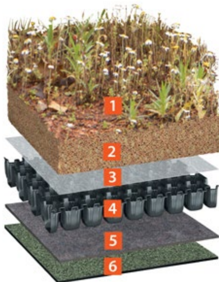
Figure 1. Typical extensive green roof build-up. (1) vegetation layer; (2) substrate layer; (3) filter fleece; (4) drainage layer; (5) protection mat; (6) waterproofing layer. © Bauder
