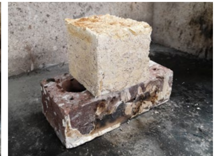
iv. Prototype 4 Date of created : 15th June 2021 Water, Lime & Bagasse Ratio : 1:1:3
