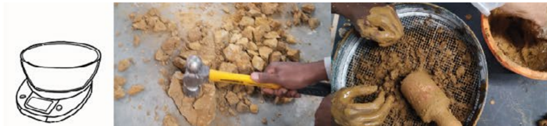
Step 2 : Prepare the material. We crushed and sift the clay for easy mixing. Prepare the materials of water, clay & bagasse.
