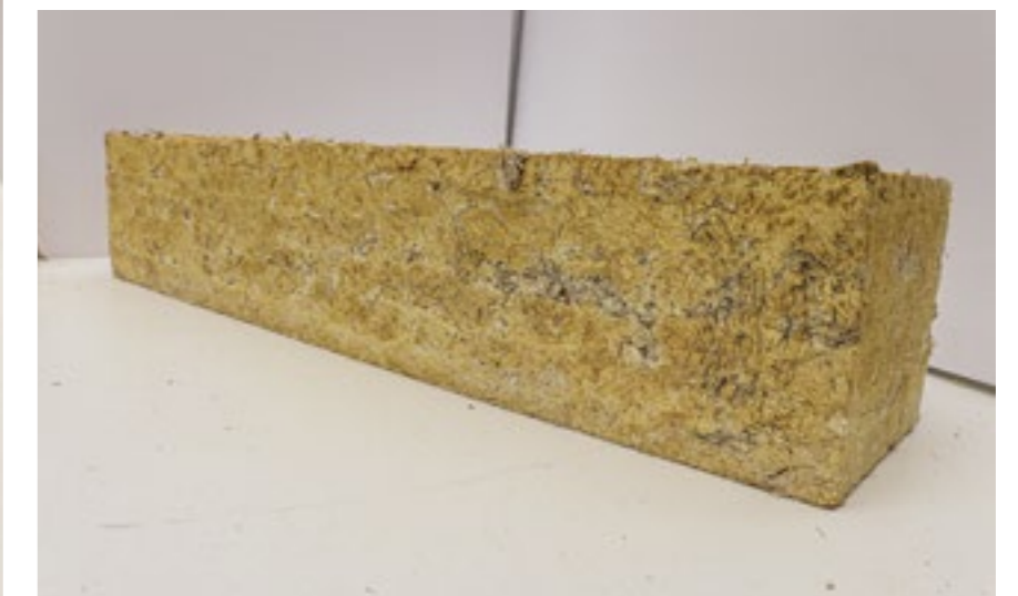
Prototype 14 - Structural Beam - 325L / 675W / 80B
