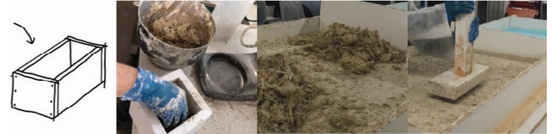
Step 4 : Pour mixture into the mold. After the mixture is mixed thoroughly, pour the mixture into the mold. Tap/press down the mixture repeatedly to have a compact panel.
