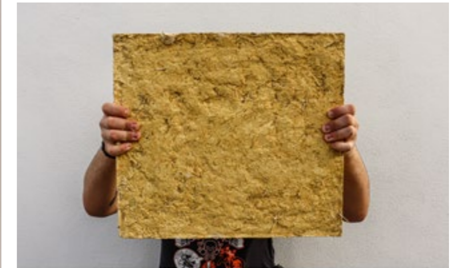
Prototype 9 - Thermal Insulation Board - 325L / 675W / 80B
