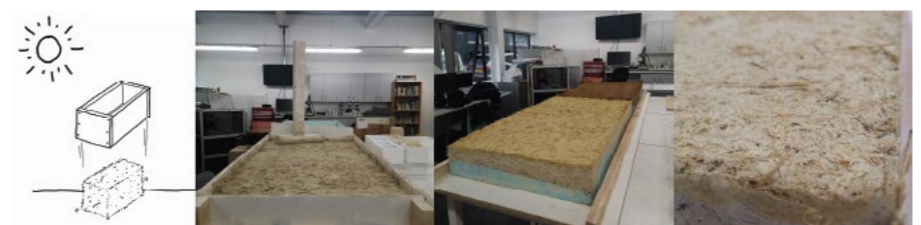
Step 5 : Let it dry. After filling up the mold up to the level needed, leave it to dry for 3 days. Afterwards, gently remove the mold from the mixture to let it dry faster.
