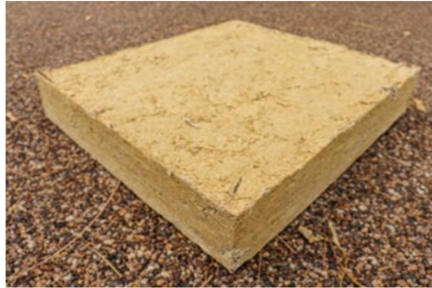
Prototype 9 - Thermal Insulation Board - 325L / 675W / 80B
