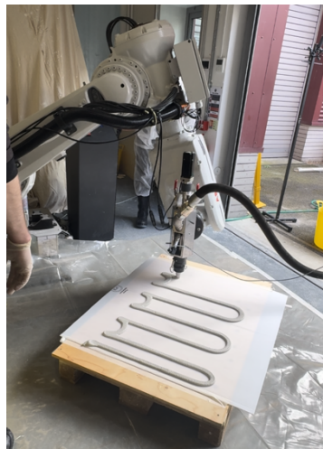
Fig. 11 Digital lab - robotic arm ABB and extrusion nozzle in testing stage
