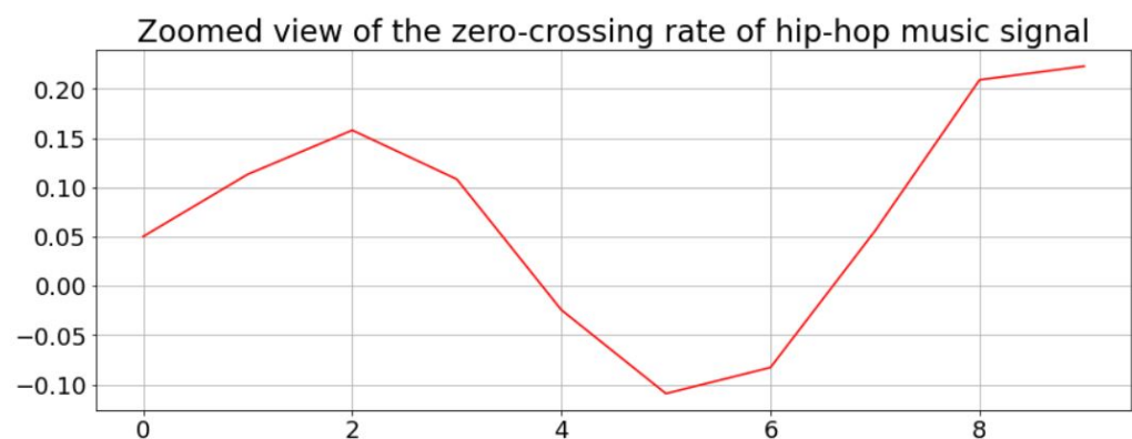
Figure 6. Zoomed view of the zero-crossing rate of hip-hop music signal for ten columns.
