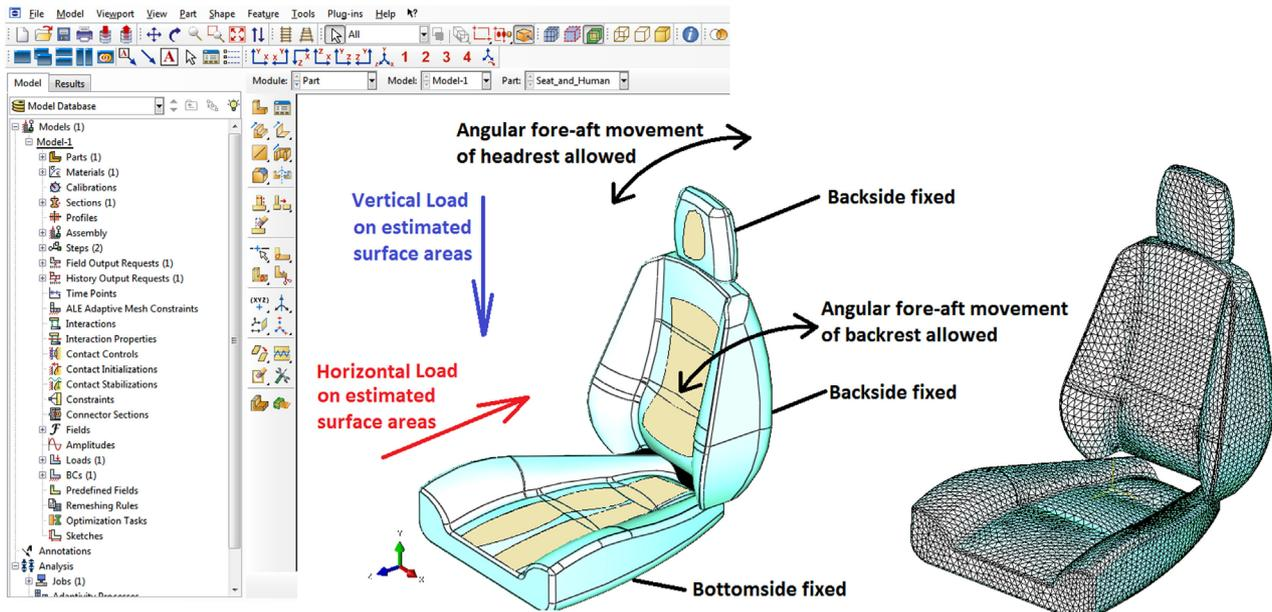
**Figure 2.** Estimated interfaces, directions of loads, boundary conditions and meshing.
