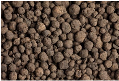
Figure 1: Lightweight coarse aggregate based on sintered fly ash (Lytag) [3]
