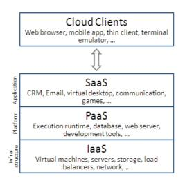
**Figure 3. Cloud Computing Layers**
