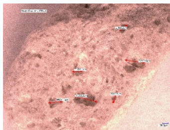
Fig. 1. Pumice aggregate porosity – optical microscopic photograph at 20x magnification
