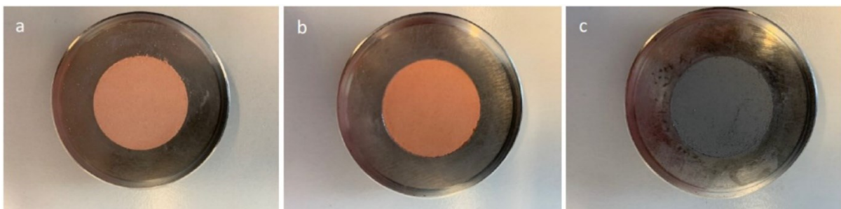
Fig. 3: Images of clay: (a) raw clay; (b) calcined clay; (c) calcined clay with colour control (Chotoli et al. 2017).
