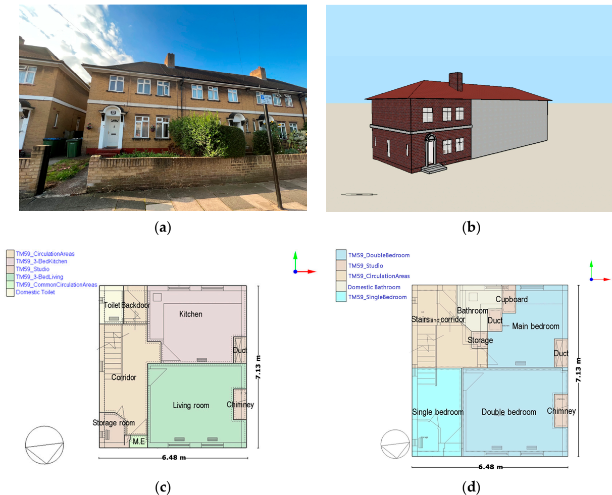
Figure 2. (a) The case study house; (b) a 3D model of the case study house; (c) ground-floor plan; (d) first-floor plan.
