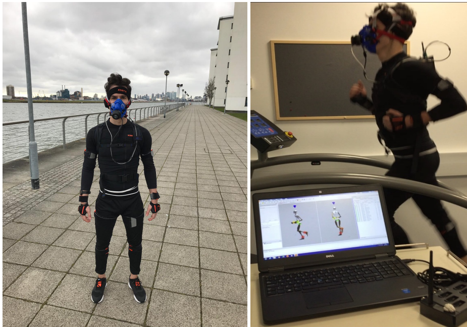
Figure 3.4: A participant demonstrates how the two data capture systems sit in unison on the body. The left picture shows the flat, straight outdoor area where the overground running took place and the right picture is in the laboratory.
