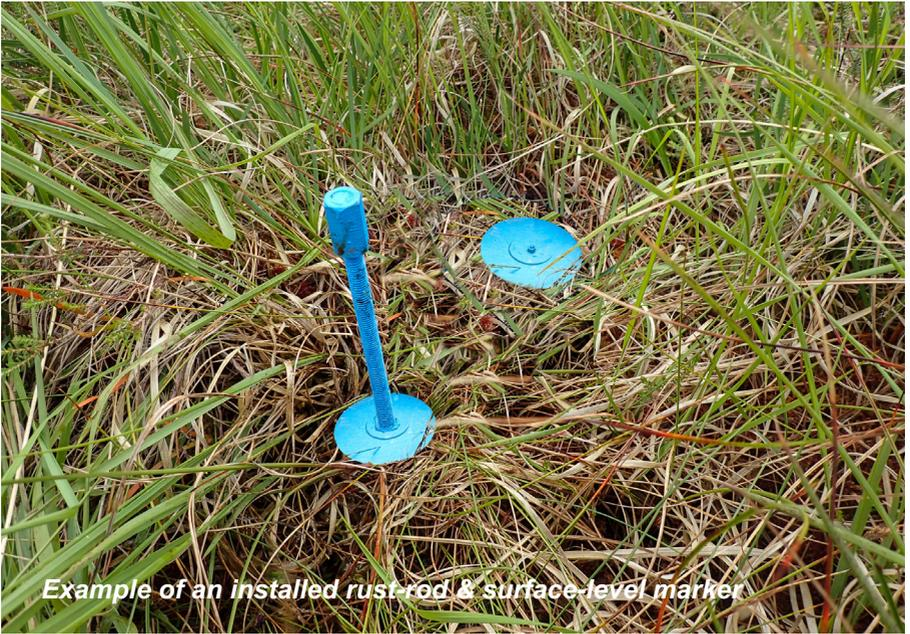
*Example of an installed rust rod & surface-level marker*
