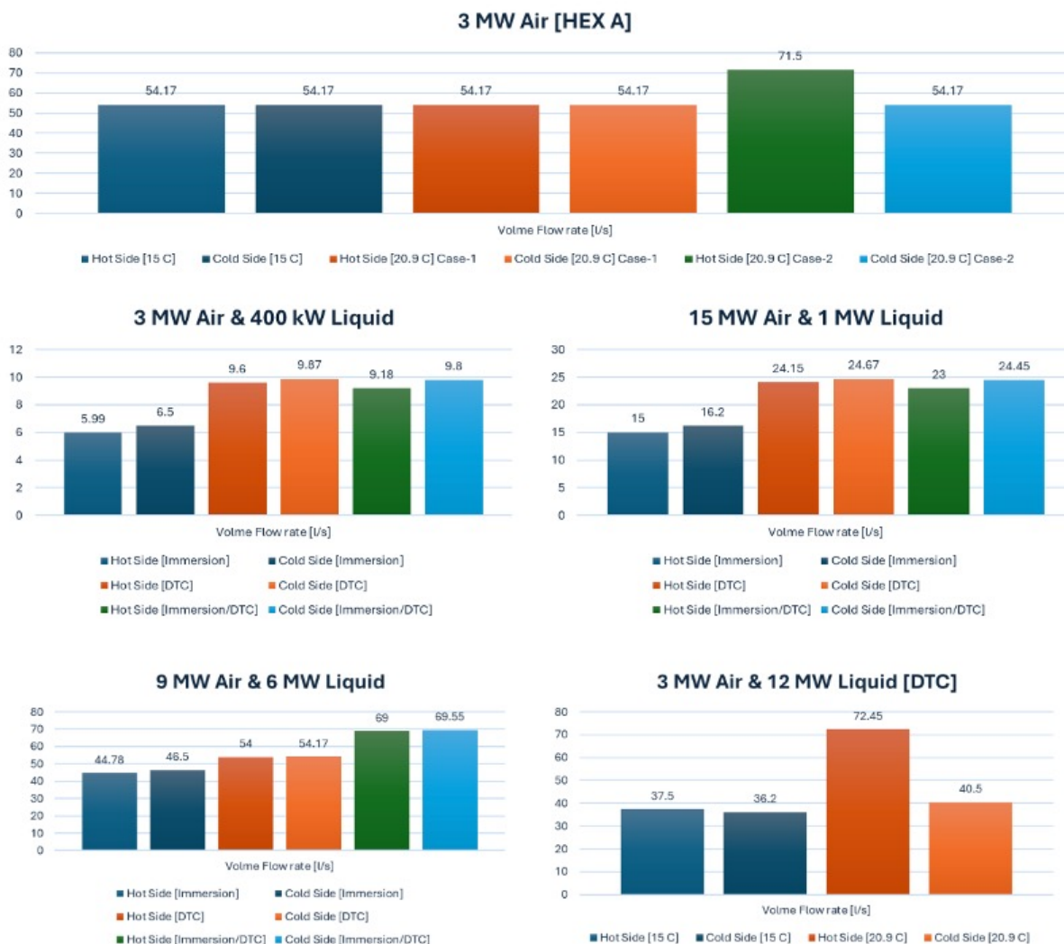
Fig. 7. Sea Water Volumetric Flow for Deployed and Proposed Case Studies.
