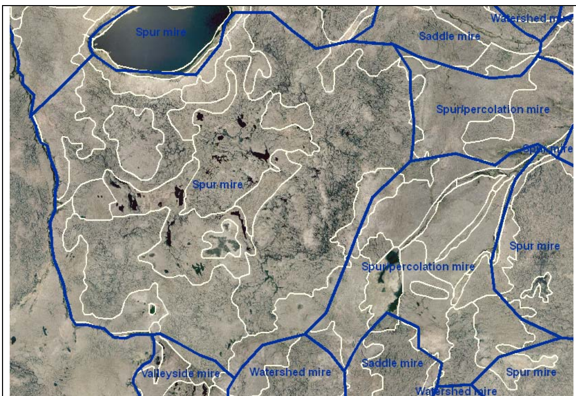
Figure 33. LWP Erosion Class boundaries as microtope boundaries. Part of the macrotope shown in Figure 31, displayed over an aerial photograph. Internal mesotope boundaries are shown and labelled (dark blue), along with pale boundaries that, in effect, delimit microtopes - regions of distinctive surface textures, whether smooth, with pools (black shapes) or complex erosion networks. Note how the surface 'texture' of the ground varies between and within mesotopes, but is largely uniform within the microtopes . This texture, or 'microtope pattern', is created by repeated arrangement of small-scale surface features such as bog pools, hummocks and hollows, and (in this case) erosion gullies.
