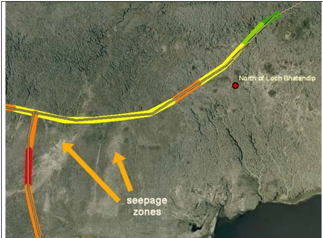
Figure 87. Peatslide issues at 'North of Loch Bhatandip'.
