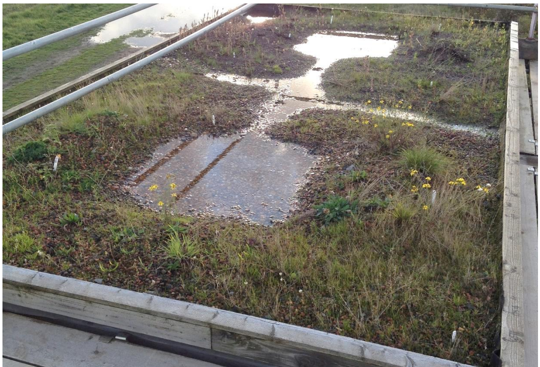
Plate 3.9. Image of (a) seasonally wet pools on an area of brownfield habitat adjacent to the green roof experiment at Barking Riverside, and (b) pools on Roof 5 with a 25 mm outlet treatment. The photos were taken on 28th October 2015 after a major rain event and shows how the design of the experimental roofs successfully mimicked the habitat character of ground-level ephemeral wetlands on site.
