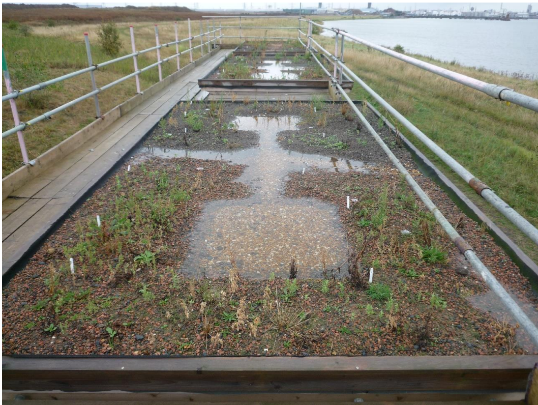
Plate 3.6. Photograph of roofs 7-9 with summer pooling taken on 26th August 2014 after heavy rainfall. Roof 7 in the foreground has 25 mm raised outlet, Roof 8 in the middle with larger pools has 50 mm outlet treatment, and Roof 9 in the background has no pooling and 0 mm outlet. A total of 34 mm of precipitation was recorded for Upminster during the previous day (IEsexUP1, www.wunderground.com ).
