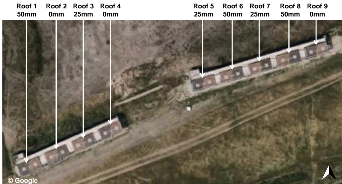
Plate 3.4. Aerial photo of the green roof experiment at Barking Riverside, East London showing randomised distribution of the three drainage test treatments. The aerial view also shows the randomisation of the east-west orientation of aggregates (brown = standard extensive, black = Lytag). Aerial image ©Google maps.
