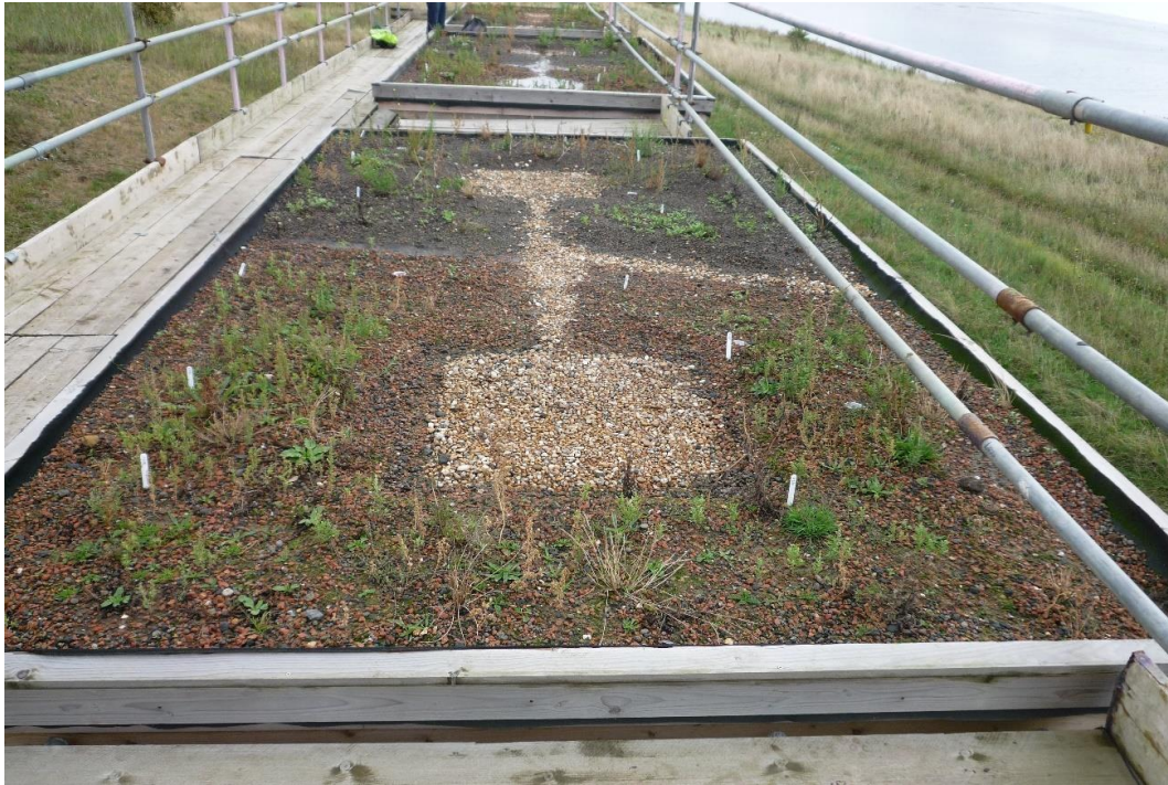
Plate 3.7. Photograph of roofs 7-9 taken on 28th August 2014, three days after heavy rainfall. Roof 7 (25 mm outlet) in the foreground no longer has pooling. Roof 8 (50 mm outlet) in the middle has much shallower pools than on 26 th August. Roof 9 (0 mm outlet) in the background has no pooling.
