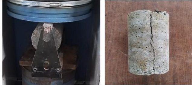
Figure 1. Condition of specimen before (a) and after (b) indirect tensile testing
