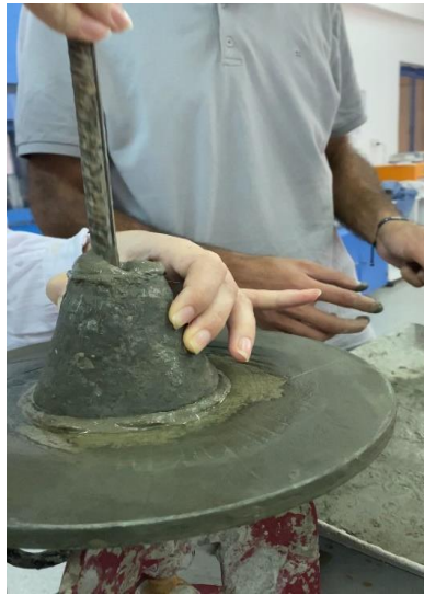
Figure 1. Placement of cement in the cone for mini slump testing
