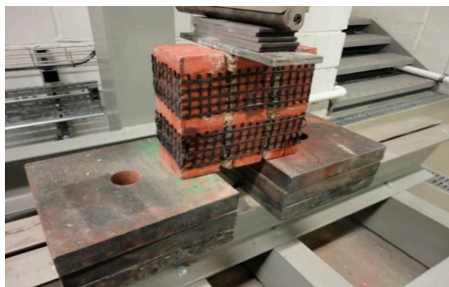
Figure 25. CFRP net strips on four sides.
