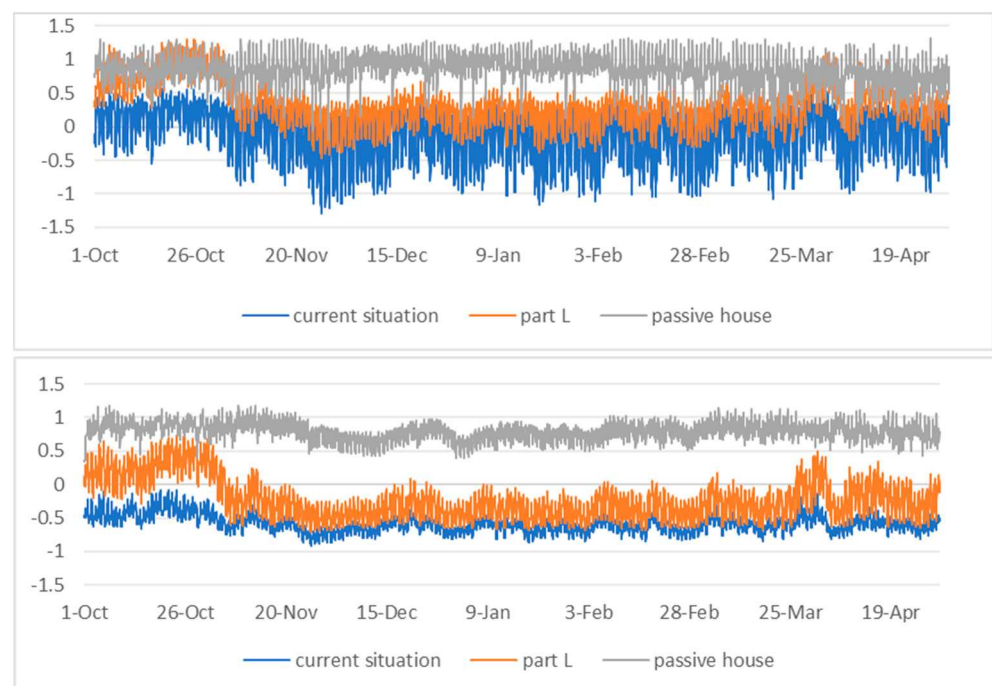
Figure 5. PMV index in (top) living room and (bottom) bedroom from October to the end of April.
