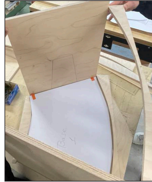
Fig. 47 - SIMULATING THE POSITION OF THE WALLS
