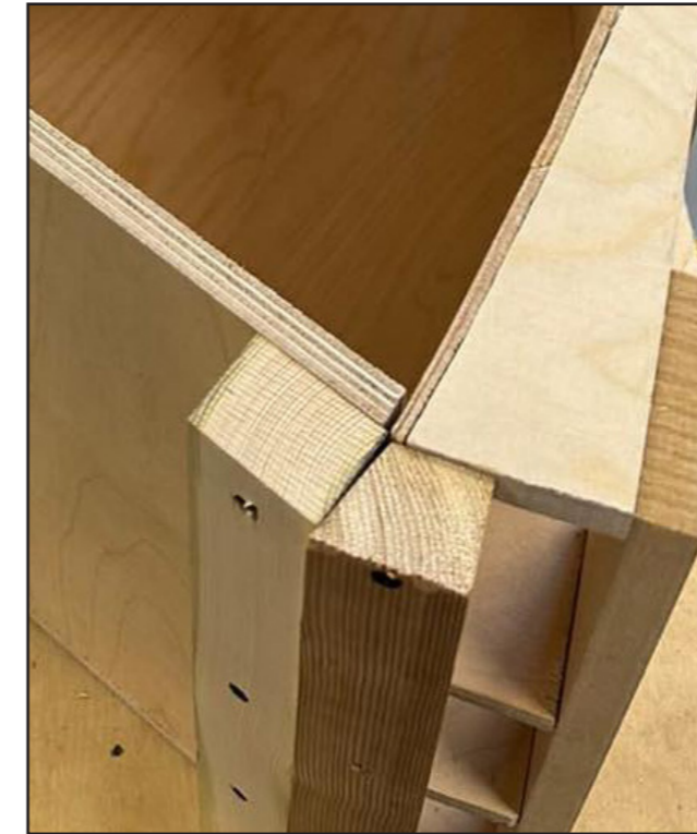
Fig. 64 - A CLOSE-UP OF THE BATTENS ALIGNED
