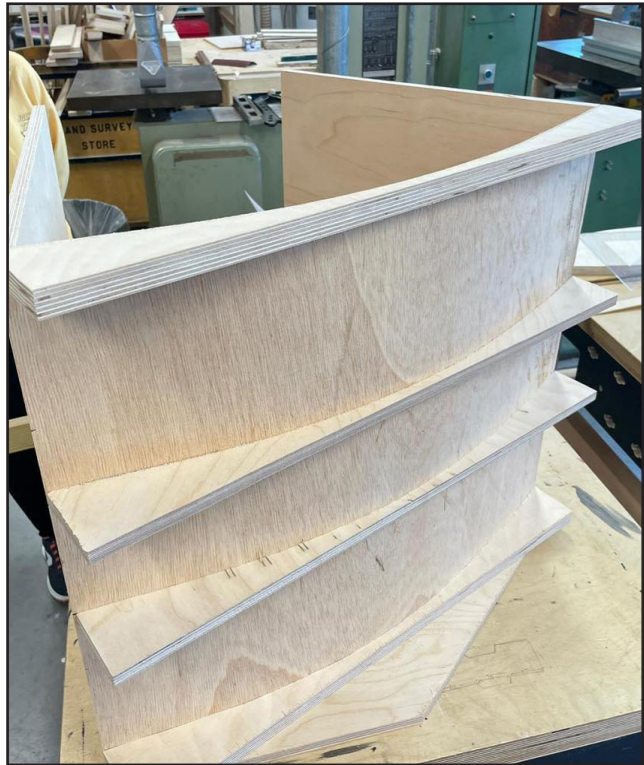
Fig. 55 - BACK VIEW OF THE FOUR RIBS MAKING THE CURVE
