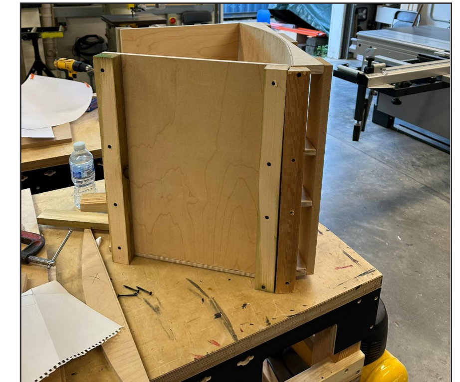
Fig. 66 - ALIGNING THE PARTS BEFORE SCREWING THEM TOGETHER
