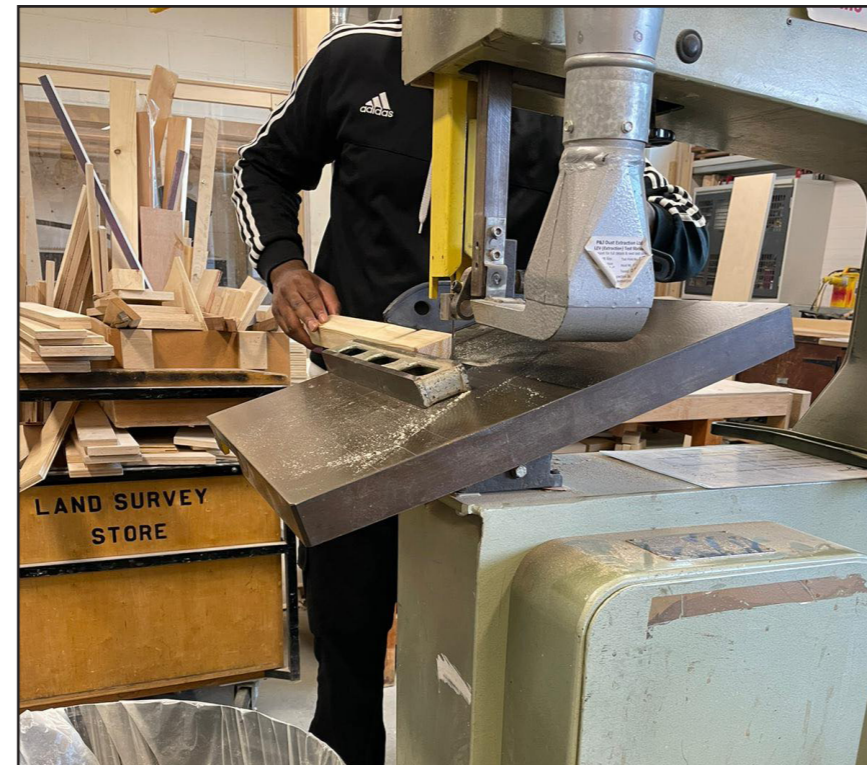
Fig. 63 - CUTTING THE BATTENS AT AN ANGLE
