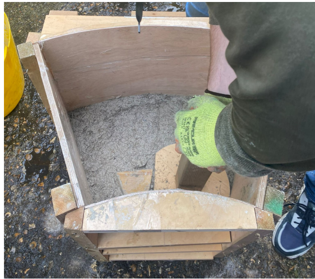
Fig.89 - COMPRESSING THE SUGARCRETE
