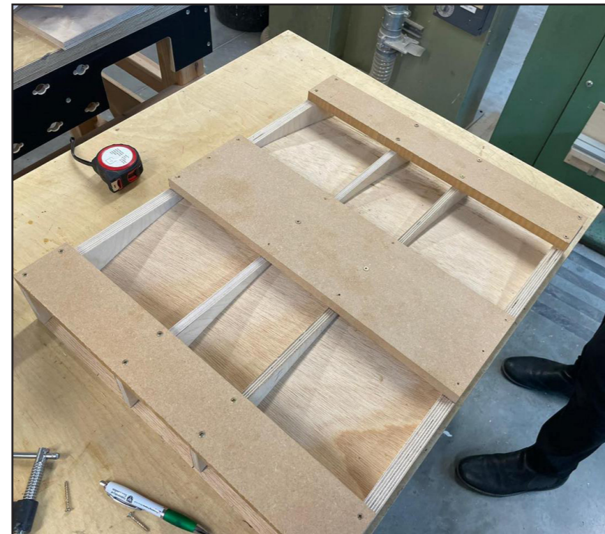
Fig. 57 - FINALISING THE REINFORCEMENT SYSTEM
