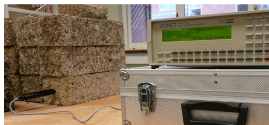
Figure 1: Testing thermal properties of blocks with an ISOMET transient heat-transfer probe.
