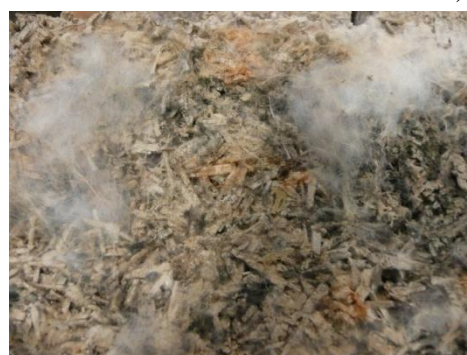
Figure 7: a) Blocks drying in the mini-greenhouse, b) mould growing on the hemp-clay-lime blocks
