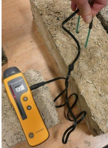
Figure 2: Measuring moisture content with a Protimeter moisture probe.
