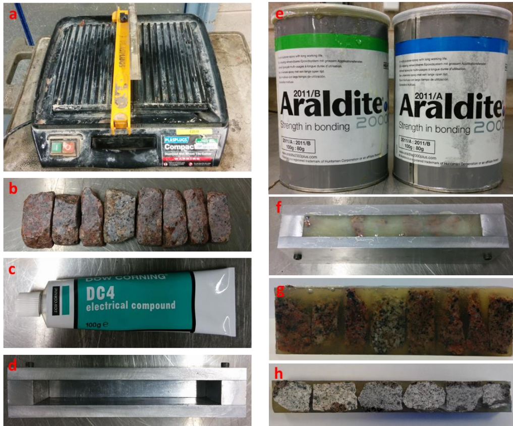
Figure 3. Procedures for aggregate substrate preparation: (a) trim saw, (b) aggregates after trimming, (c) release compound, (d) assembled mould, (e) epoxy resin, (f) combine trimmed aggregates in the mould and fill the gaps with epoxy resin, (g) cured composite aggregate, (h) composite substrate used for peel test.
