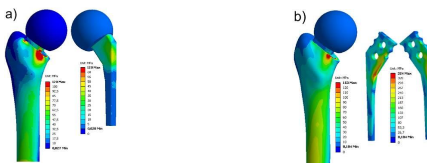
Figure 4. Equivalent von Mises stress distribution. a) Non-Reinforced Spacer at F_R = 3000\text{ N} ; b) Endoskeleton Including Spacer at F_R = 5000\text{ N} (Thielen et al., 2009)
