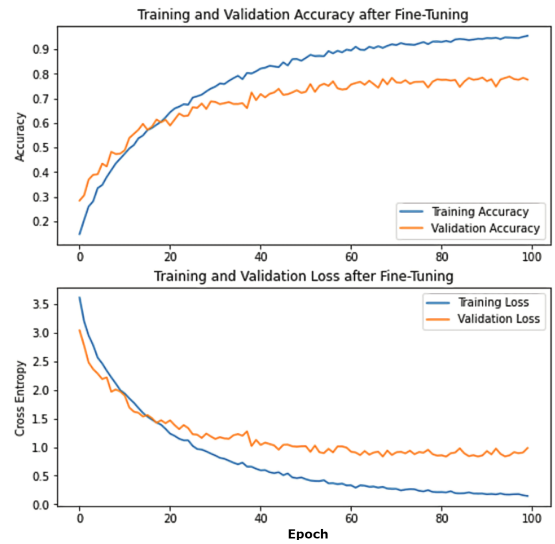
Fig. 12. MobileNet-V1 accuracy and loss curves after fine-tuning with 0.6 dropout rate only.
