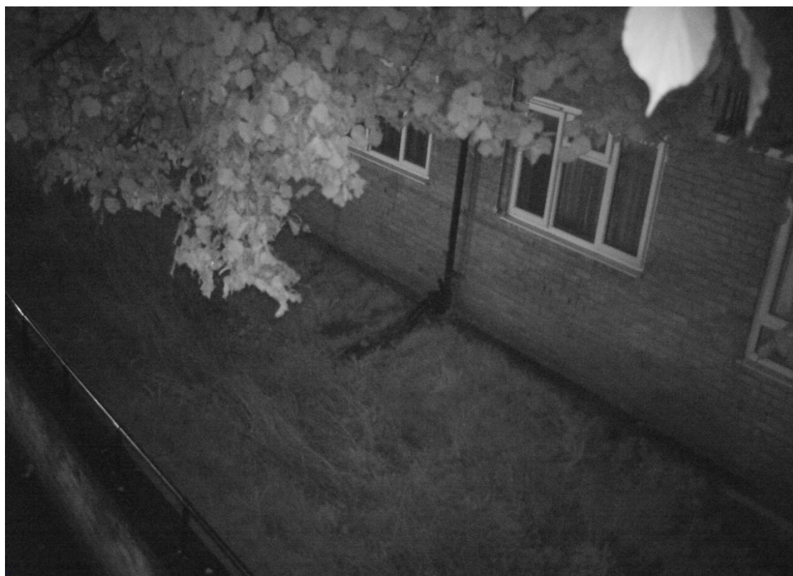
Figure 21. Time-lapse camera images from Beatrice House swale (FPC4), 09/08/2017. Images show i) no evidence of overflowing during a period of high rain intensity at 10:36 and ii) evidence of 100% infiltration/conveyance by the end of the intense rain event at 23:54 on the same day.
