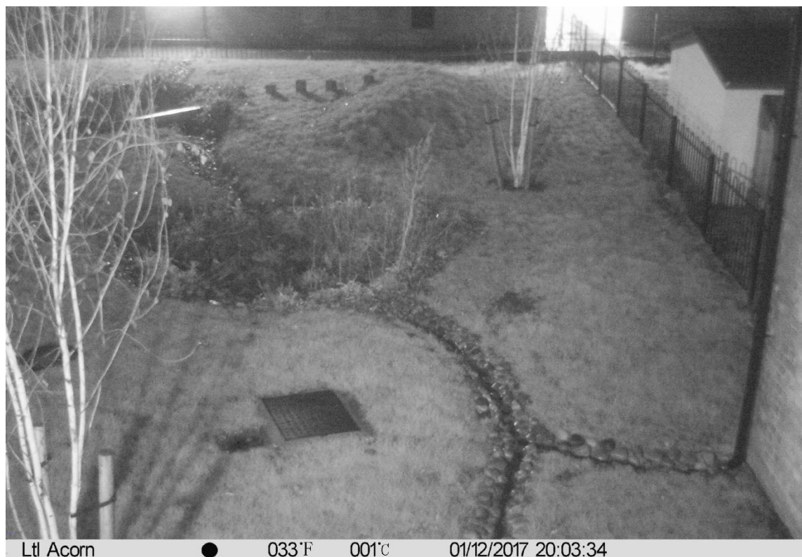
Figure 118. Time-lapse camera images from Community Hall and Sofia House basins (FPC2), 12/01/2017. Images show i) no evidence of overflowing during a period of high rain intensity at 17:22 and ii) evidence of 100% infiltration/conveyance by the end of the intense rain event at 20:03 on the same day.
