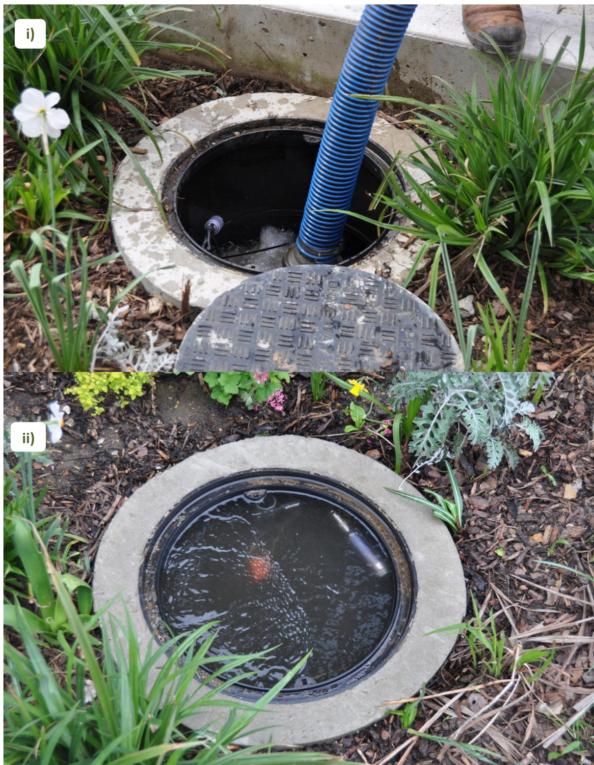
Figure 71. Images from the storm simulation event at the Sun Road rain gardens, Cheeseman Terrace Estate, 24th March 2017. Images show i) water being pumped into the inspection chamber of the rain garden; ii) inlet chamber full after the stormwater was pumped in.
