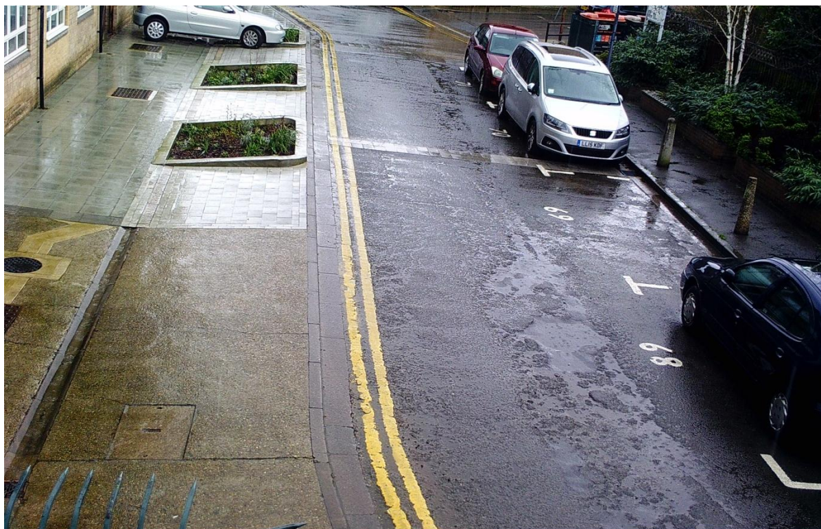
Figure 133. Time-lapse camera images from Cheeseman Terrace rain gardens (FPC6), 27/02/2017. Images show i) no evidence of overflowing during the first period of high rainfall at 03:37 and ii) evidence of 100% infiltration/conveyance during the second, more intense, rain event at 10:22 on the same day.
