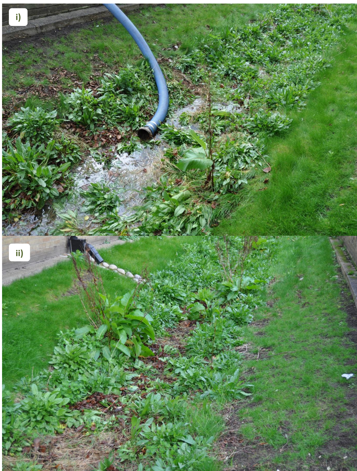
Figure 66. Images from the storm simulation event at Beatrice House swale, Queen Caroline Estate, 23rd March 2017. Images show i) the Beatrice House swale immediately after the last of the 10,000 Litres of water was released and ii) the centre of the swale where the water was pumped in 10 minutes after the last of the water was released.
