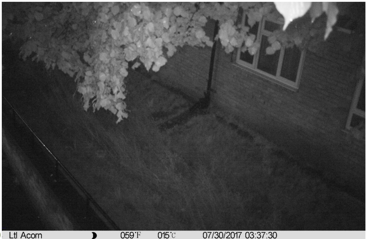
Figure 140. Time-lapse camera images from Beatrice House swale (FPC4), 30/07/2017. Images show i) no evidence of overflowing during a period of high rain intensity at 02:29 and ii) evidence of 100% infiltration/conveyance by the end of the intense rain event at 03:37 on the same day.
