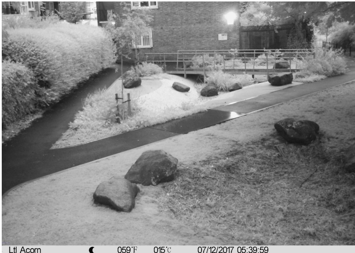
Figure 155. Time-lapse camera images from Adella House grass and stoney basins (FPC3), 22/07/2017. Images show i) no evidence of overflowing during a period of high rain intensity at 19:54 on the 11th and ii) evidence of 100% infiltration/conveyance by the end of the intense rain event at 05:39 on the 12th.
