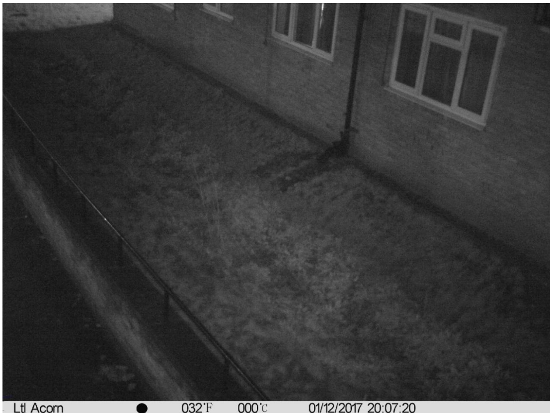
Figure 120. Time-lapse camera images from Beatrice House swale (FPC4), 12/01/2017. Images show i) no evidence of overflowing during a period of high rain intensity at 16:34 and ii) evidence of 100% infiltration/conveyance by the end of the intense rain event at 20:07 on the same day.
