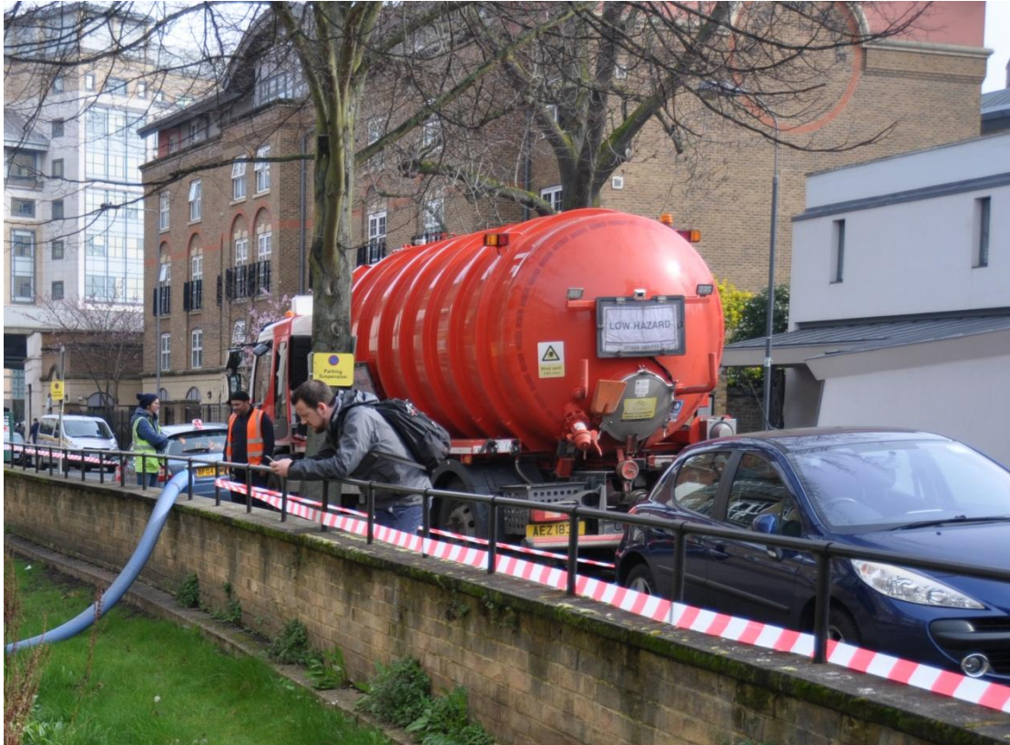
Figure 62. Water tanker delivering 10,000 Litres of non-potable water for the storm simulation event at Beatrice House swale. Storm simulation was carried out over the course of an hour on the 23rd March 2017.
