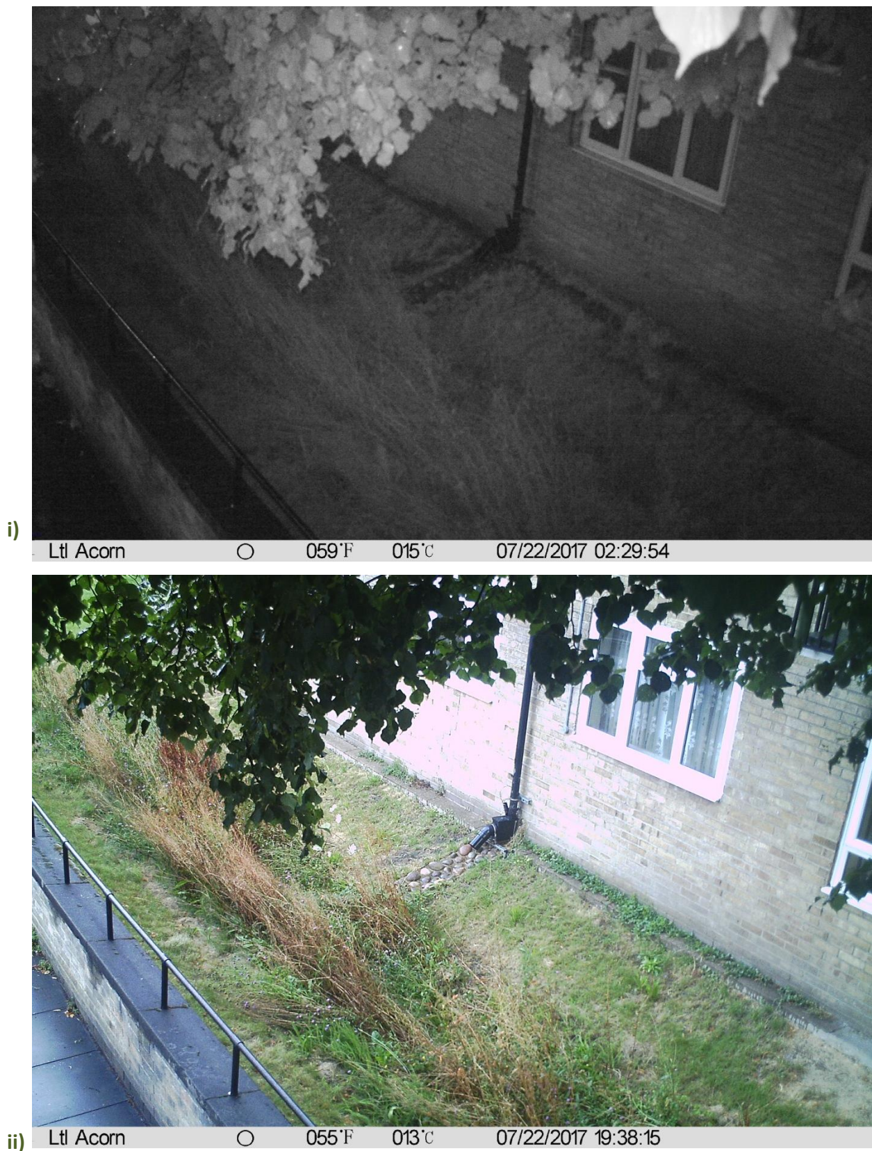
Figure 148. Time-lapse camera images from Beatrice House swale (FPC4), 22/07/2017. Images show i) no evidence of overflowing during a period of high rain intensity at 02:29 and ii) evidence of 100% infiltration/conveyance by the end of the intense rain event at 19:38 on the same day.
