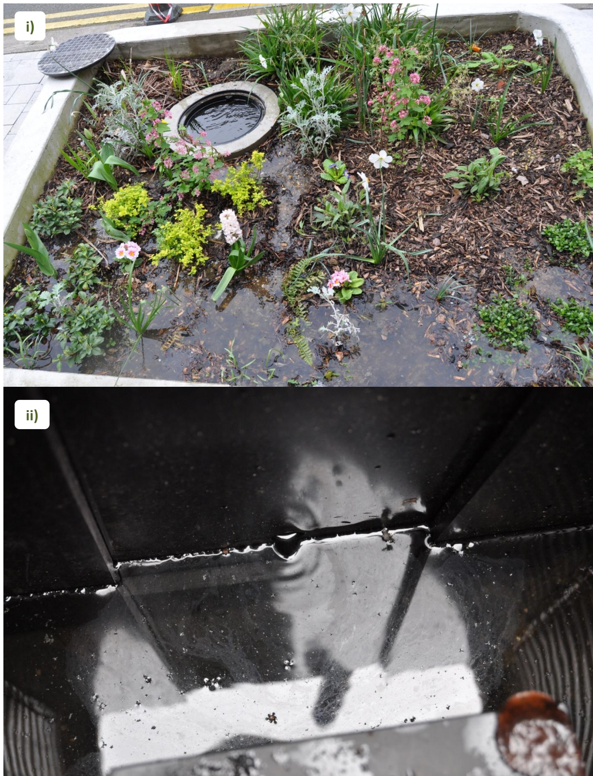
Figure 72. Images from the storm simulation event at the Sun Road rain gardens, Cheeseman Terrace Estate, 24th March 2017. Images show i) the rain garden inspection chamber overflowing onto the rain garden during the rain simulation and ii) the control flow chamber releasing water from the rain gardens following the 1 in 5 year storm event simulation.
