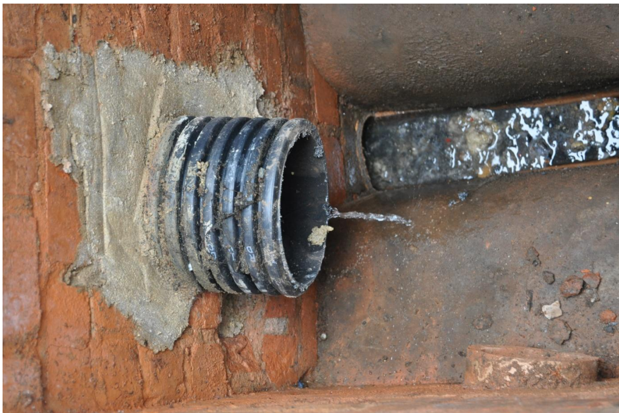
Figure 73. Image from the storm simulation event at the Sun Road rain gardens, Cheeseman Terrace Estate, 27th March 2017. Image shows the stormwater that was released from the rain garden overflow being released to the combined sewer system during the final 1000 L release of the stormwater simulation test.
