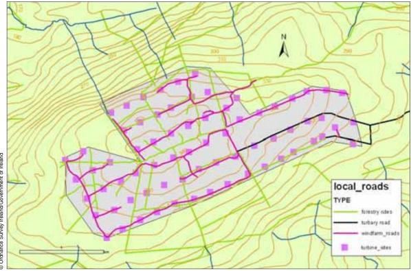
Figure 5.2: Arrangement of existing turbary road (black) and forest rides (green) on the Derrybrien site together with the new floating roads (purple) built before October 2003. (New roads according to AGEC 2004.) Some of the turbine sites (lilac squares) are not yet served by access roads so that a need for further road construction can be anticipated. Stream-courses are shown in blue, contours in pale brown.
