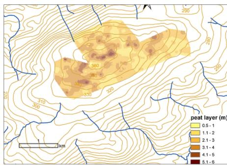
Figure 2.1: The depth of peat recorded for Cashlaundrumlahan within the area of development. Surface contours give some indication of slope, while the streamlines indicate patterns of drainage.
