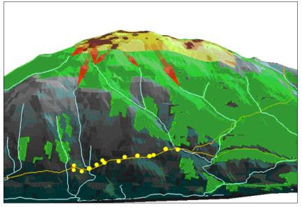
Figure 10.2a, above left: Three-dimensional view of the Cashlaundrumlahan summit from the WNW. It shows showing the extent of forestry (green shading), streamcourses (blue), roads (brown) and the depth of peat in the wind farm
