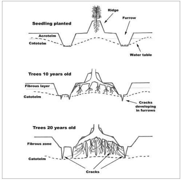
Figure 3.1: The sequence of drying and cracking that occurs in peat over a 20-year period beneath plantation forestry, particularly when the crop is lodgepole pine, *Pinus contorta* (adapted from Pyatt 1987).
