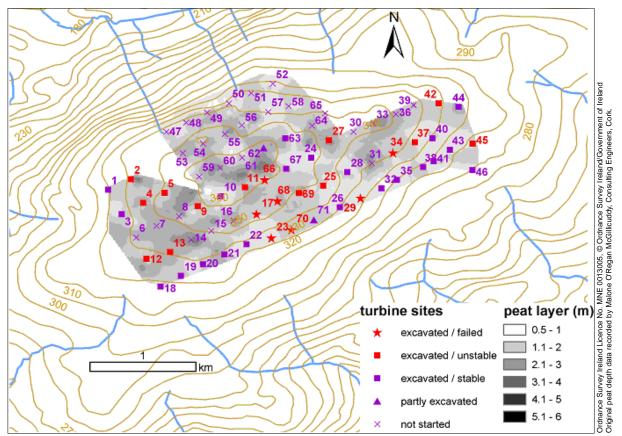
Figure 9.1: Summary of the stage and stability of turbine excavations from AGEC (2004). Unstable excavations are those where localised cracking or slumping has occurred. Sites marked as failed are those where downslope movement of peat has occurred or where incipient rotational failures were recorded.
