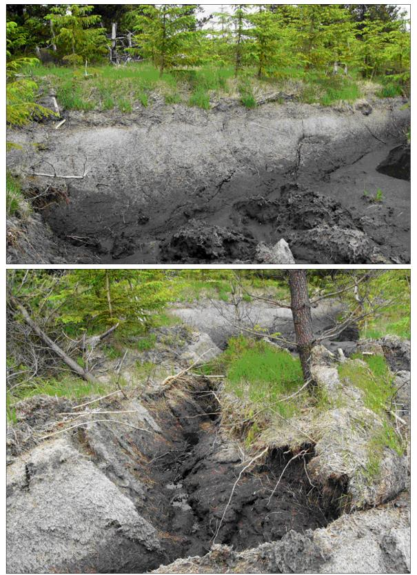
Plate 8.7: Delaminated ribbons of peat at the edge of the failed area near T70. The two-layered structure of the peat profile is obvious on the faces of the ribbons but there are few protruding tree roots. Some cracking of catotelm peat is evident in the upper picture.
