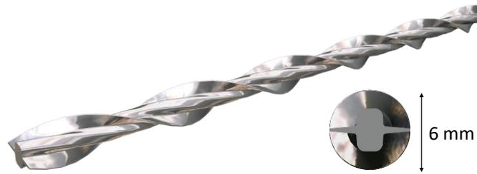
**Fig. 7.** Geometry of the helical bars
