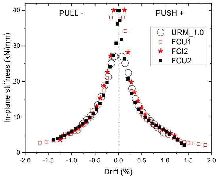
**Fig. 15.** Typical degradation of in-plane stiffness.
