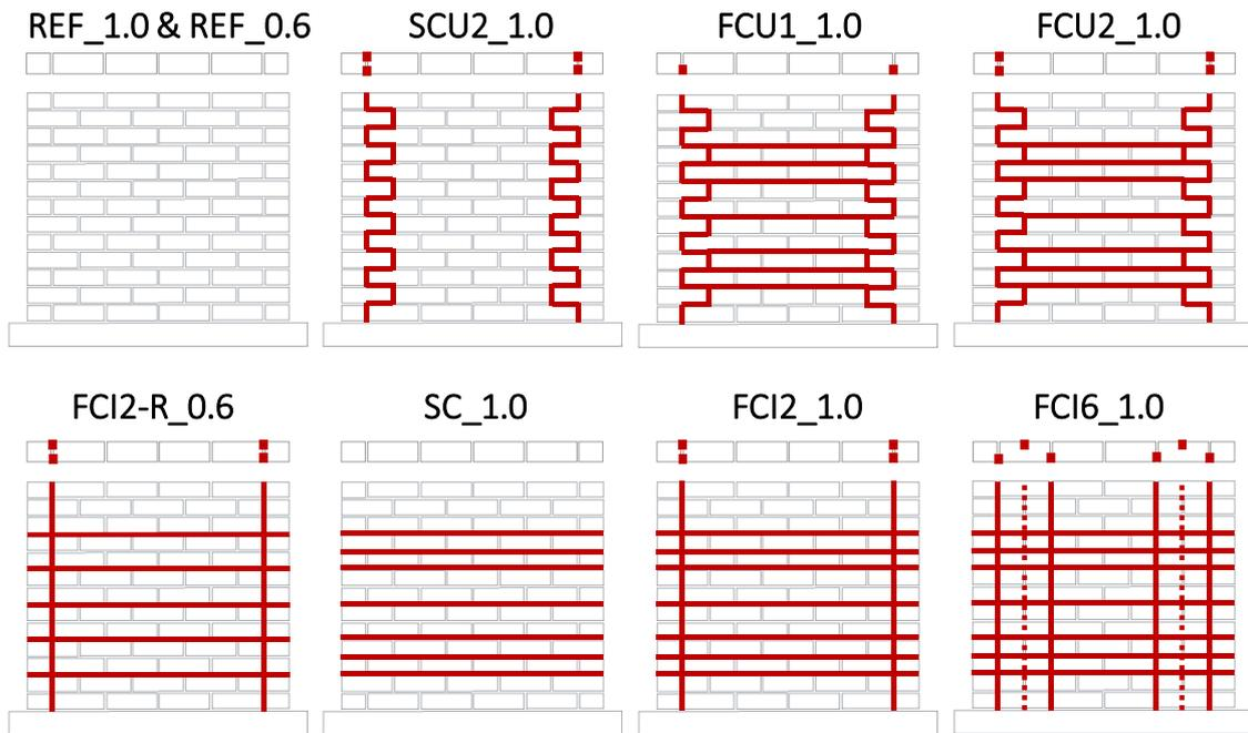
\*Note that all vertical bars were fitted into the PFC adapter prior casting concrete infill to achieve full anchorage in the base.
