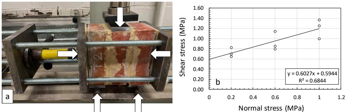
**Fig. 6.** Initial shear strength – test rig and results: a) test rig; b) test results for all 9 triplets
