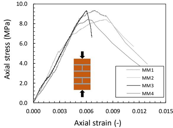
**Fig. 5.** Compressive characteristics of masonry brick-mortar assemblages.
