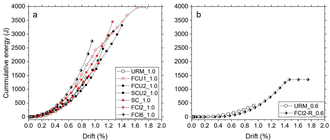
**Fig. 17.** Energy dissipation for increasing drift levels: a – walls specimens with an axial stress level of 1.0 MPa; b – walls with an axial stress level of 0.6 MPa.
