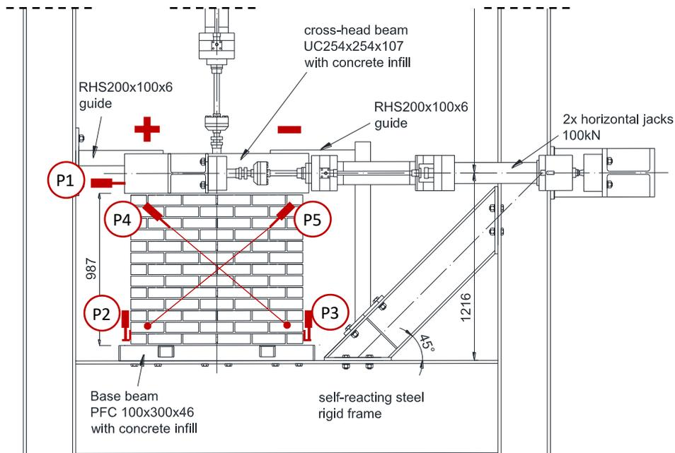
**Fig. 11.** Test setup and instrumentation – frontal elevation. Note that diagonal gauges were installed on the back side of the wall. The signs “+” and “-“ indicate directions of loading – push and pull, respectively.
