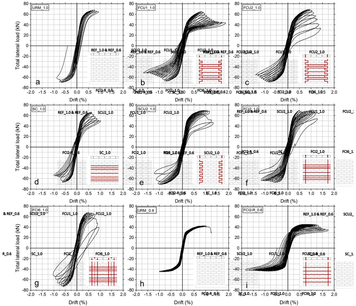
Fig. 14. Load-drift hysteresis loops for all walls.
