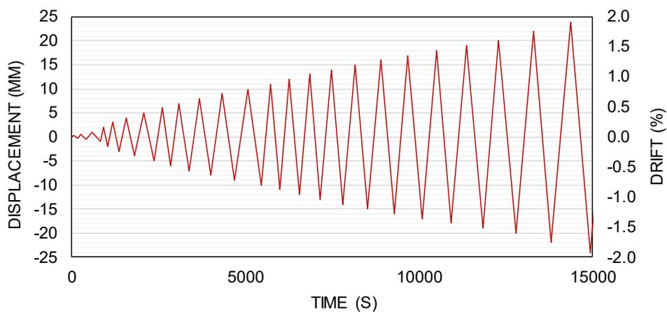
**Fig. 12.** Loading protocol adopted for the in-plane cyclic shear testing.
