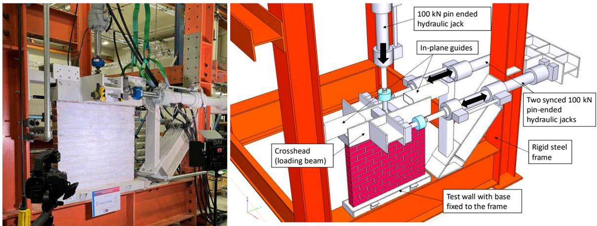
**Fig. 10.** Typical test setup for in-plane testing with cyclic reversals.
