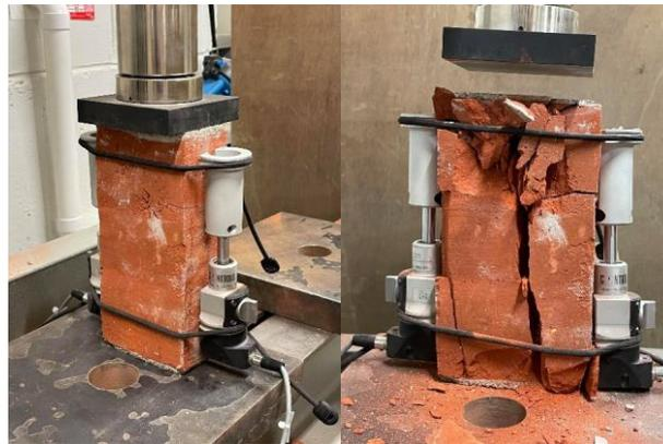
**Fig. 3.** Masonry unit tested under compression before and after failure.
