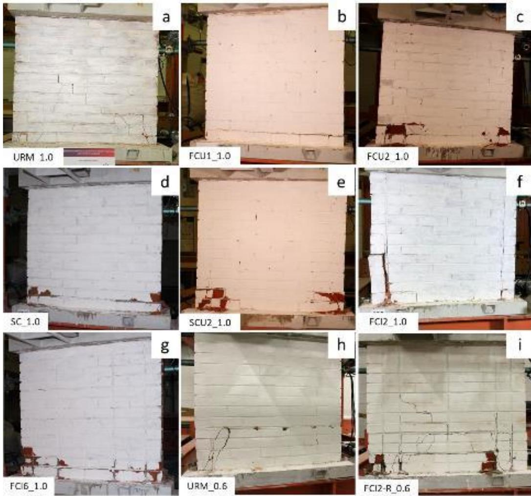
**Fig. 13.** Failure patterns for all walls.
