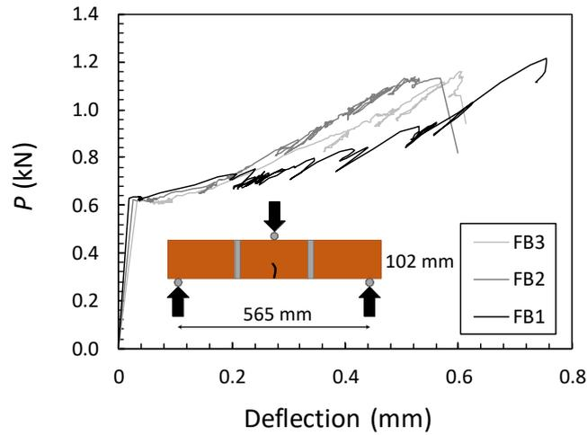
**Fig. 4.** Three-point bending test on brick-mortar assemblages.
