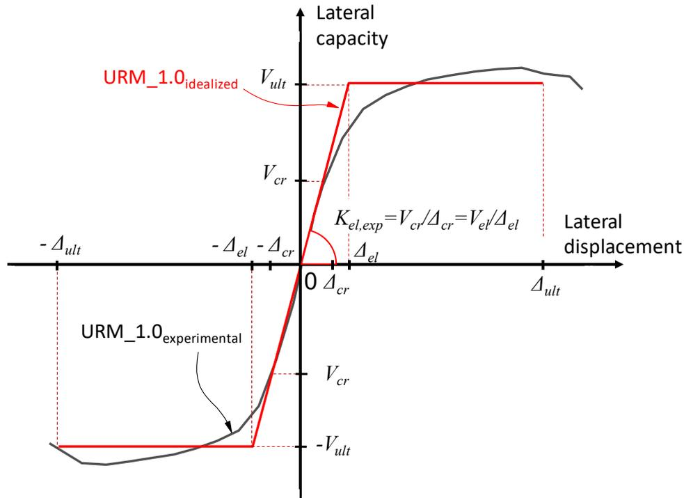
**Fig. 16.** Typical bilinear idealisation of force-displacement response.
