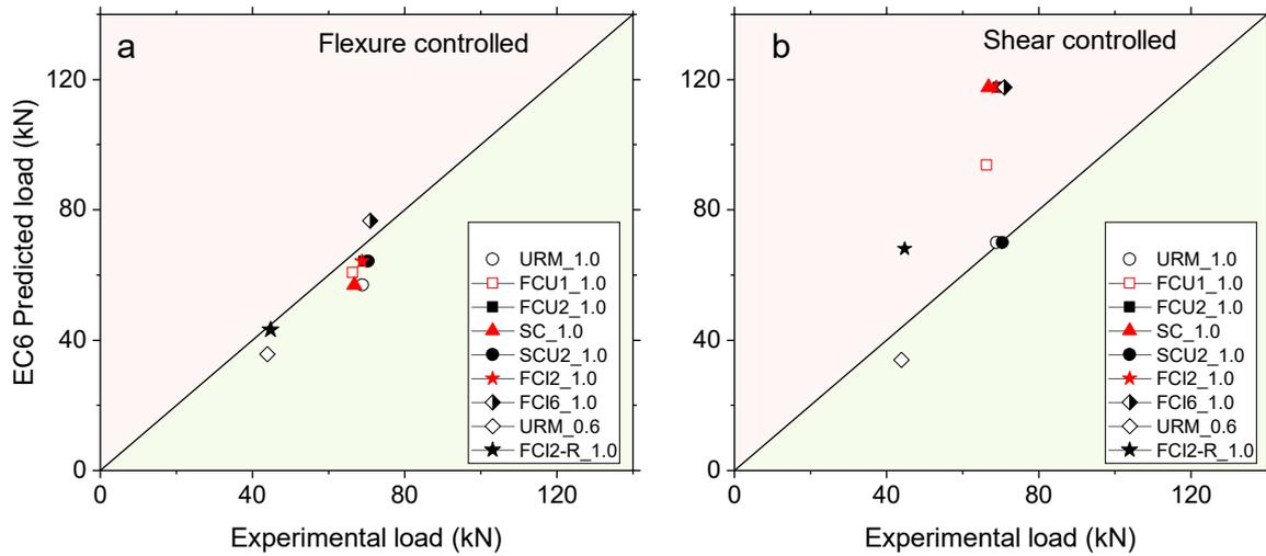
**Fig. 18.** Predictions of lateral load capacity: a – Predictions associated with flexural failure; b – predictions associated with shear failure.
