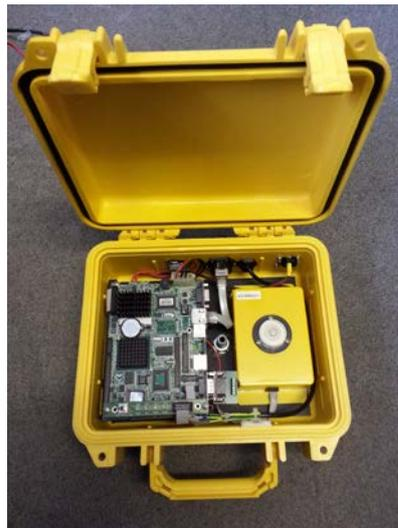
**Figure 1: CUSP 3B Digital Accelerograph, Canterbury Seismic Instruments Ltd**
