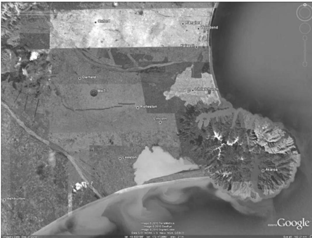
▲ **Figure S4.** Aerial shot of the Christchurch area showing the surface fault rupture and the epicentre of the Darfield EQ the image is about 117 km across.
