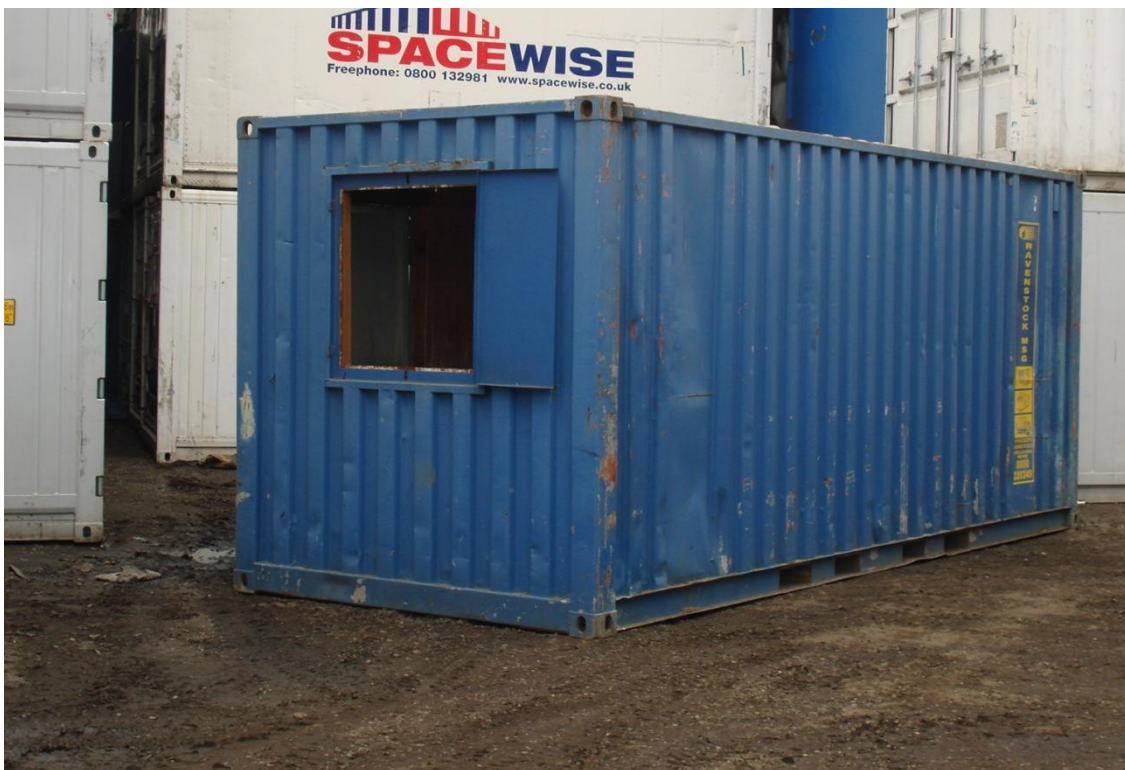
Figure 5. One of nine scrap 20 ft freight containers for the Phase 2 green roof experimental treatments at Barking Riverside, East London. It was possible to source old damaged containers at a discounted price as these were not suitable for further use for freight transportation.
