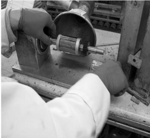
**Fig. 2.72.** Application of glue to the rotor stack.
