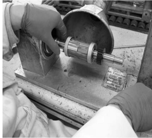
**Fig. 2.73.** Insertion of permanent magnets to the rotor stack.
