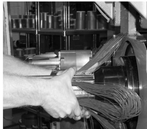
**Fig. 2.51.** Winding preparation.
