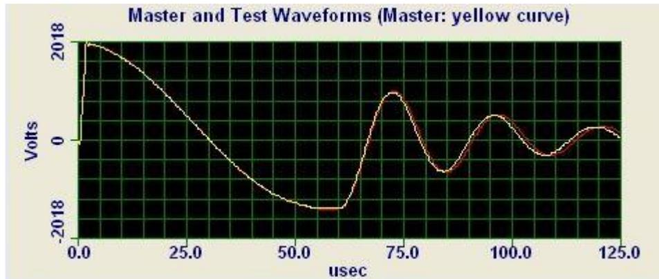
Fig. 6.10. Paper wall insulation Material D flash test.
